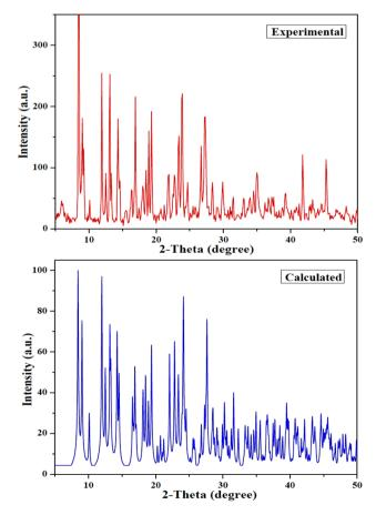
Fig. 11 Experimental (top, red) and calculated (bottom, blue) XRD pattern of  $[Zn(HL)(OAc)_2]$ .
