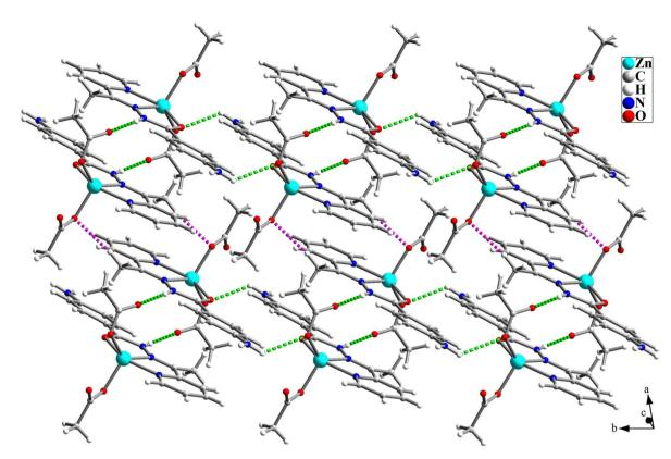
Fig. 3 Hydrogen bond interactions  $(N-H\cdots O = \text{green and } C-H\cdots O = \text{pink})$  in the structure of  $[Zn(HL)(OAc)_2]$  (1)
