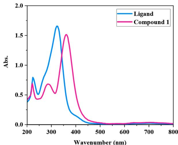
Fig. 6 UV-vis spectra of HL and [Zn(HL)(OAc)<sub>2</sub>] ( $2.5 \times 10^{-5}$  M) in methanol.
