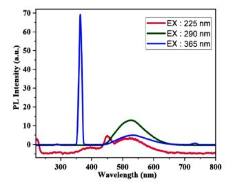
Fig. 7 The PL spectra of  $[Zn(HL)(OAc)_2]$  at the different excitation wavelengths.
