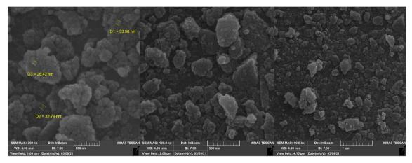
Fig. 10 SEM images of the heterogeneous catalyst (Si-[Zn(HL)(OAc)<sub>2</sub>]).
