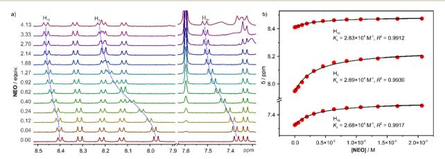
Fig. 4 (a) Partial <sup>1</sup>H NMR spectra (500 MHz, CD<sub>2</sub>Cl<sub>2</sub>, 298 K) of H1 titrated with different concentrations of NEO. (b) The non-linear fitting of three proton signals against concentrations of NEO using a 1:1 binding model.
