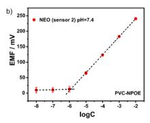
Fig. 5 (a) Response of EMF to incremental changes in the **NEO** concentration. (b) Calibration curves of the **H1**-based electrode to **NEO**
