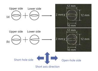
Fig. 6 Exoskeleton frames used in Experiment 1. (a) The exoskeleton having a symmetrical hole. (b) The exoskeleton having an asymmetrical hole.
