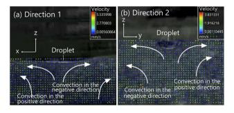
Fig. 11 Convection generated around a droplet, under the condition of using the aqueous solution with a concentration of 0.5 mL/100 mL of water and the symmetrical exoskeleton. (a) Convection captured from Direction 1. (b) Convection captured from Direction 2.
