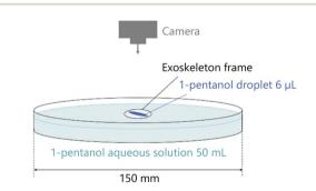
Fig. 3 Experimental setup of the preliminary experiment
