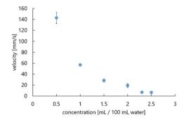
Fig. 4 Relationship between concentration of aqueous solution and average velocities of self-propelled droplets.
