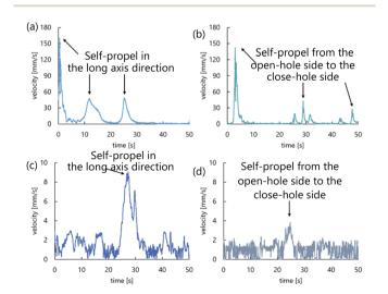
Fig. 8 Time evolution of the self-propulsion velocity. (a) 0.5 mL/100 mL water, the symmetrical exoskeleton. (b) 0.5 mL/100 mL water, the asymmetrical exoskeleton. (c) 2.3 mL/100 mL water, the symmetrical exoskeleton. (d) 2.3 mL/100 mL water, the asymmetrical exoskeleton.
