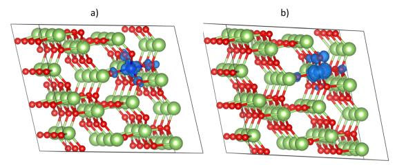
Fig. 3 Diagram of (a) Ni and (b) Ir substitution at  $Ga_2$  site. The green and red balls represent  $Ga_2$ ,  $Ga_2$ , respectively. The blue lobes show the localization of electron (a)  $Ni_{Ga_2}^{0}$  and (b)  $Ir_{Ga_2}^{1+}$  in the spin-singlet state.
