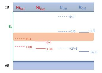
Fig. 2 The schematic band diagram illustrates the defect-level energies for Ni<sub>Ga</sub> and Ir<sub>Ga</sub> defects. The shaded orange row indicates the estimated Fermi-energy range.
