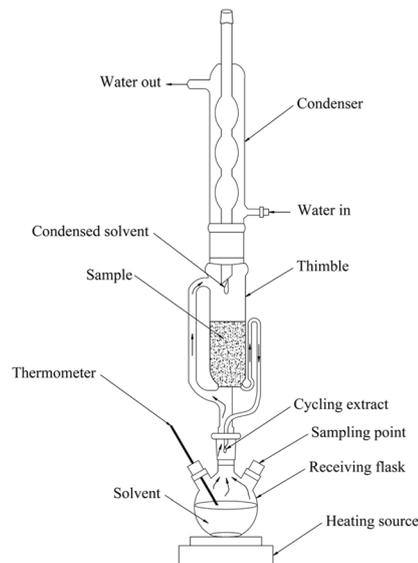
Fig. 1 Scheme of Soxhlet apparatus.
