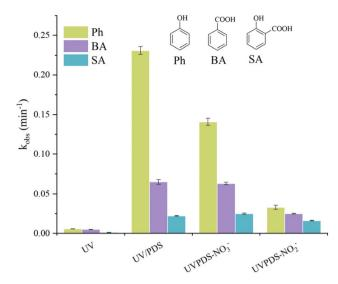
Fig. 1 Removal rate of the 3 compounds in various processes (conditions: [Ph] = [BA] = [SA] = 0.1 mM, [PDS] = 0.5 mM,  $[NO_3^-]$  = 2 mM,  $[NO_2^-]$  = 2 mM, pH = 3, T = 60 min).
