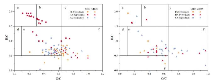
Fig. 5 Van Krevelen diagrams of byproducts from oxidation of Ph, BA and SA under the influence of  $NO_3^-$  (left) and  $NO_2^-$  (right).
