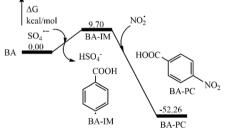
Fig. 4 Energy change in the reaction of the target pollutants and radicals at/B3LYP/6-31+G(d) level under SMD model (IM for intermediate, TS for transition state, and PC for principal component).
