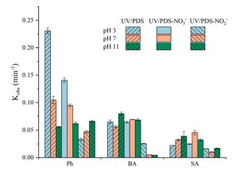
Fig. 2 Effect of pH on reaction rate of the 3 compounds (conditions: [pollutant] =  $0.1 \, \text{mM}$ , [PDS] =  $0.5 \, \text{mM}$ , [NO<sub>3</sub><sup>-</sup>] =  $2 \, \text{mM}$ , [NO<sub>2</sub><sup>-</sup>] =  $2 \, \text{mM}$ ,  $T = 60 \, \text{min}$ ).
