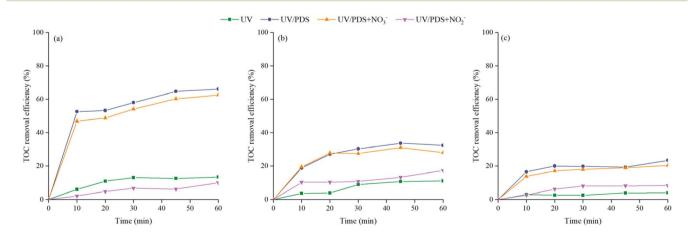
Fig. 3 Effect of  $NO_3^-/NO_2^-$  on TOC removal in UV/PDS with Ph (a), BA (b) and SA (c) as the target pollutant (condition: [pollutant] = 0.1 mM,  $[PDS] = 0.5 \text{ mM}, [NO_3^-] = 2 \text{ mM}, [NO_2^-] = 2 \text{ mM,pH} = 3).$
