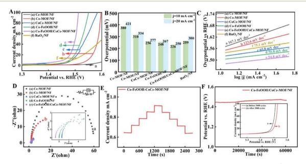
Fig. 5 Electrocatalytic performance evaluation for OER. (A) LSV curve. (B) Comparison of overpotential at 10 and 20 mA cm<sup>-2</sup>. (C) Tafel plots. (D) EIS spectra. (E) Multistep chronopotentiometry at different current densities. (F) Chronopotentiometry curves at 10 mA cm<sup>-2</sup>.
