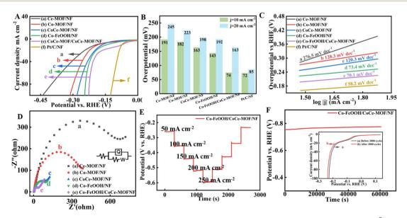
Fig. 6 Electrocatalytic performance evaluation for HER. (A) LSV curve. (B) Comparison of overpotential at 10 and 50 mA cm<sup>-2</sup>. (C) Tafel plots. (D) EIS spectra. (E) Chronopotentiometry curves at 10 mA cm<sup>-2</sup>. (F) Multistep chronopotentiometry at different current densities.
