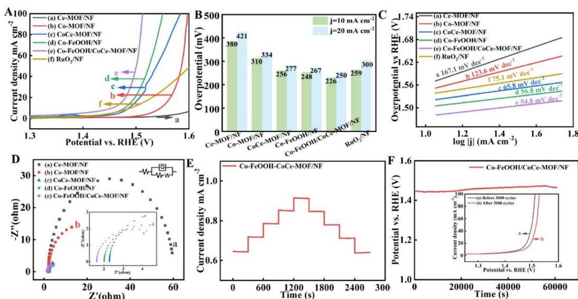
Fig. 5 Electrocatalytic performance evaluation for OER. (A) LSV curve. (B) Comparison of overpotential at 10 and 20 mA cm<sup>-2</sup>. (C) Tafel plots. (D) EIS spectra. (E) Multistep chronopotentiometry at different current densities. (F) Chronopotentiometry curves at 10 mA cm<sup>-2</sup>.
