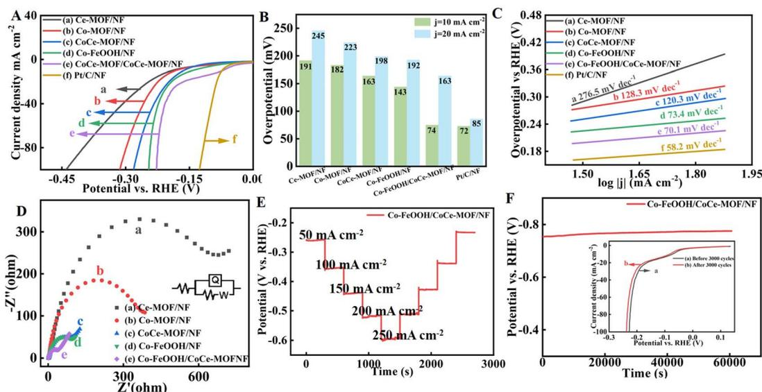
Fig. 6 Electrocatalytic performance evaluation for HER. (A) LSV curve. (B) Comparison of overpotential at 10 and  $50 \text{ mA cm}^{-2}$ . (C) Tafel plots. (D) EIS spectra. (E) Chronopotentiometry curves at  $10 \text{ mA cm}^{-2}$ . (F) Multistep chronopotentiometry at different current densities.
