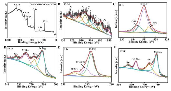
Fig. 4 XPS investigation of the Co-FeOOH/CoCe-MOF/NF sample: (A) survey spectrum, (B) Ce 3d, (C) O 1s, (D) Fe 2p, (E) C 1s and (F) Co 2p.
