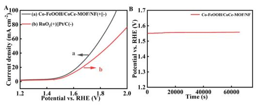
Fig. 7 (A) Comparison in 1 M KOH for various electrocatalysts. (B) Stability testing of Co-FeOOH/CoCe-MOF/NF catalyst for overall water splitting performance conducted in 1 M KOH.
