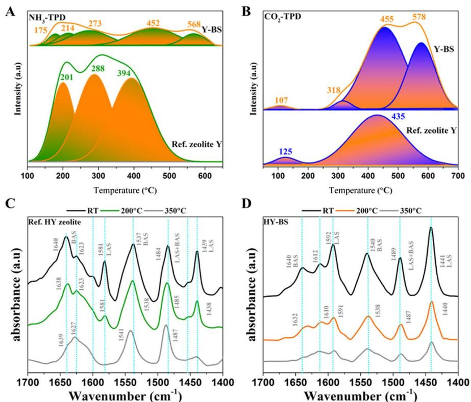
Fig. 2 (A) NH<sub>3</sub>-TPD and (B) CO<sub>2</sub>-TPD spectra of the reference HY zeolite and the HY-BS, (C and D) Py-IR of the reference HY zeolite and the HY-BS.
