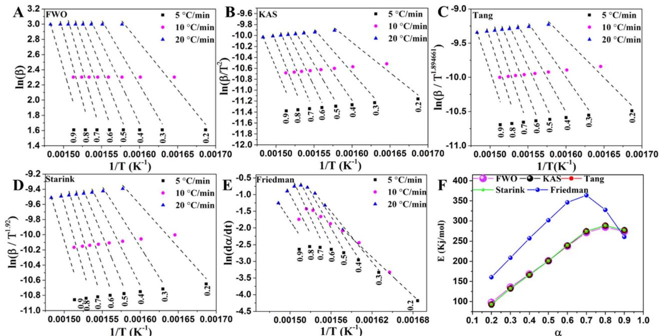
Fig. 7 The linear fitted curves were obtained from (A) FWO, (B) KAS, (C) Tang, (D) Starink, and (E) Friedman methods and (F) variation of activation energy *versus* conversion level using these methods for catalytic cracking of LLDPE in the presence of HY-BS.
