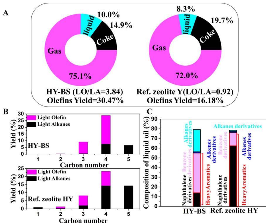
Fig. 3 Yield (%) of (A) total gas, liquid, and coke, (B) light olefins and light alkanes components of the gas fractions, and (C) and liquid oil components obtained from LLDPE cracking by the HY zeolite and HY-BS.
