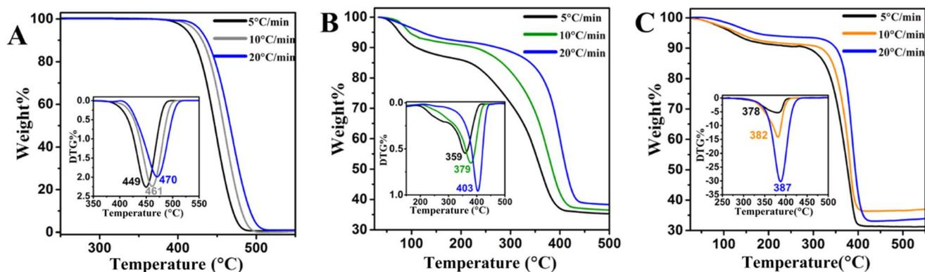
Fig. 4 TGA and dTGA of LLDPE decomposition of (A) sole LLDPE, (B) LLDPE + HY zeolite, and (C) LLDPE + HY-BS at heating rate of 5, 10, and 20 °C min<sup>-1</sup>. The weight ratio of LLDPE and zeolite was 60 : 40.
