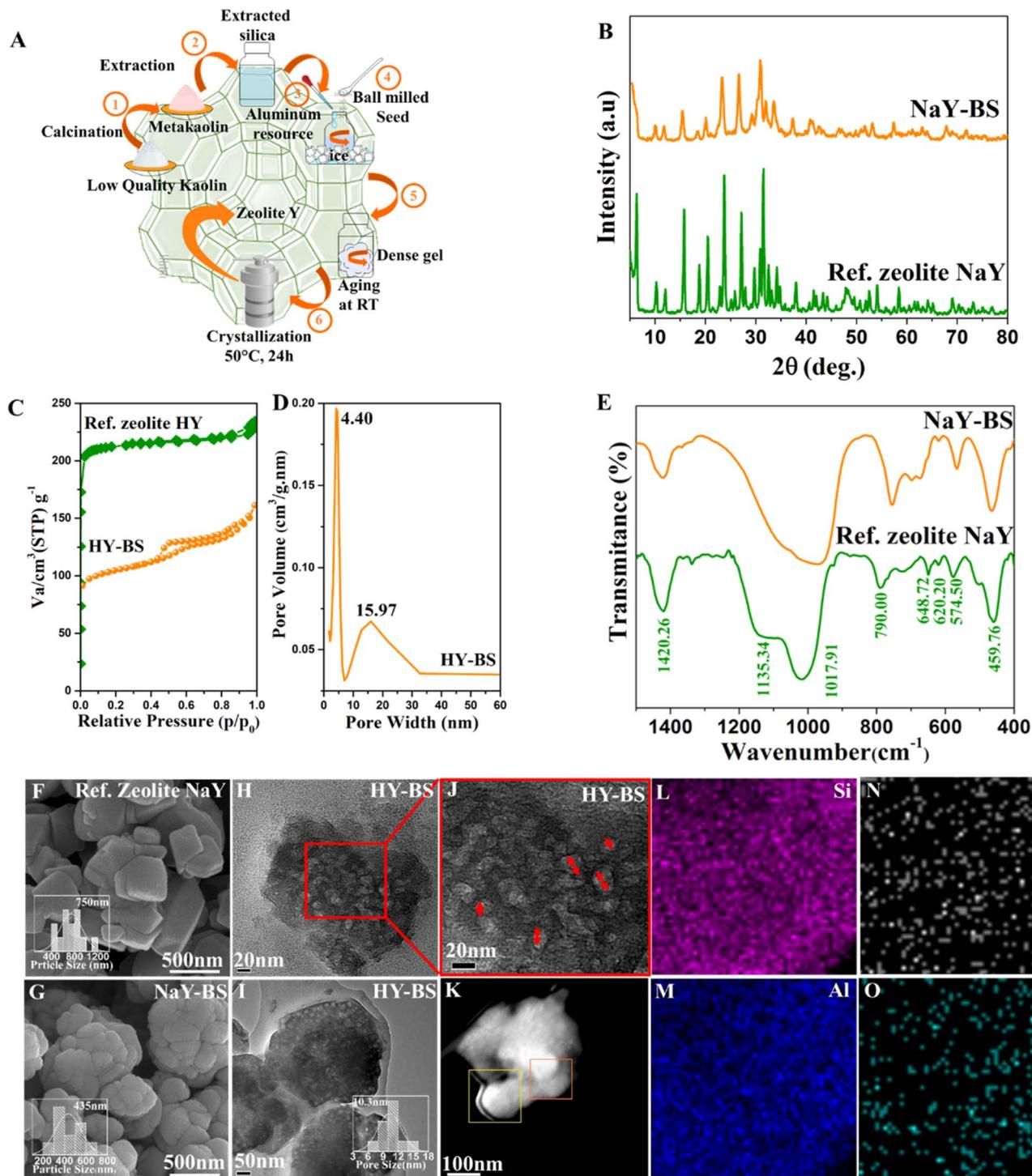
**Fig. 1** (A) Schematic of the procedure of NaY-BS synthesis, (B) XRD patterns, (C)  $N_2$  sorption isotherms of the reference HY zeolite and HY-BS, (D) pore size distribution, (E) FTIR spectra, (F and G) FE-SEM images of the reference NaY zeolite and NaY-BS, (H–J) HRTEM study of microtomed cross-section of HY-BS shown in different magnification, and (K–O) TEM-EDS mapping of the HY-BS. The double-headed arrows indicate mesopores.
