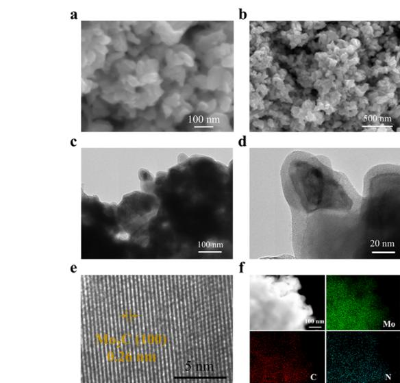
Fig. 3 (a) and (b) FESEM images, (c–e) TEM and HRTEM images and (f) EDS color mapping images of Mo<sub>2</sub>C/CN-850.
