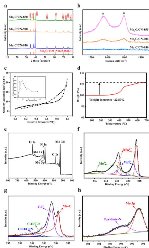
Fig. 2 (a) XRD pattern, (b) Raman spectrum of Mo<sub>2</sub>C/CN-850, Mo<sub>2</sub>C/CN-900 and Mo<sub>2</sub>C/CN-950 (c) N<sub>2</sub> adsorption/desorption isotherms curve, the inset is pore size distribution, (d) TGA curve, (e) XPS survey spectrum, and (f) Mo 3d, (g) C 1s, (h) N 1s XPS high-resolution spectra of Mo<sub>2</sub>C/CN-850.
