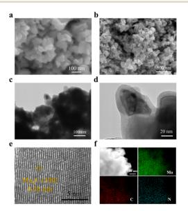
Fig. 3 (a) and (b) FESEM images, (c–e) TEM and HRTEM images and (f) EDS color mapping images of  $Mo_2C/CN-850$ .
