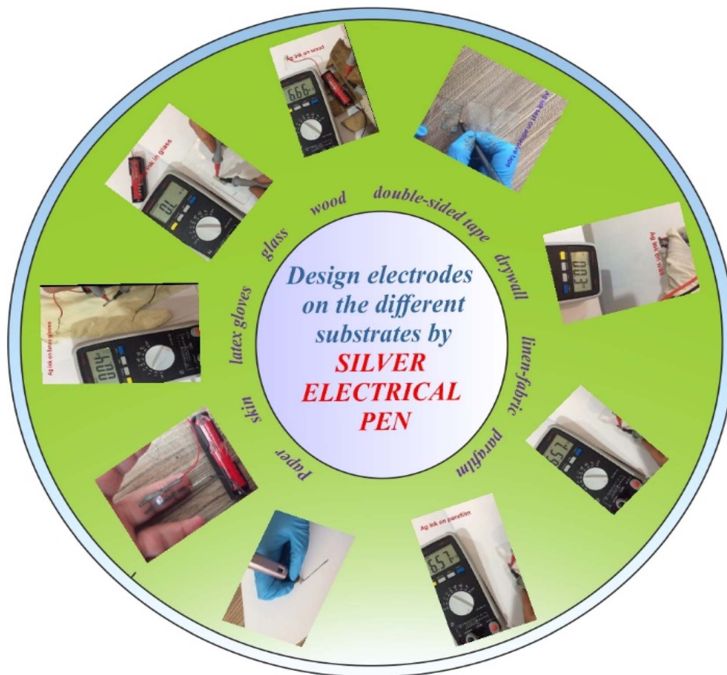
Scheme 3 Design electrodes on the different substrates by silver electrical pen.
