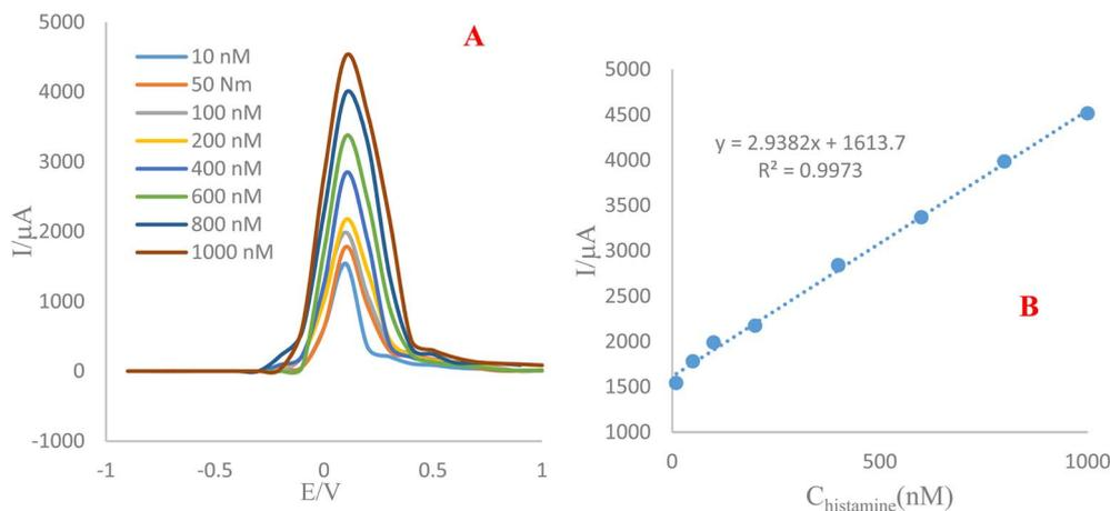
Fig. 7 (A) SWVs of the engineered sensor in different concentrations of histamine biomarker (10, 50, 100, 200, 400, 600, 800 and 1000 nM). (B) Relationship between  $I_{pa}$  and histamine concentration in meat sample.  $T_{eq} = 2$ ,  $E_{begin} = -1$  V,  $E_{end} = 1$  V,  $E_{step} = 0.1$  V, amplitude = 0.001 V, frequency = 10 Hz. Using  $K_3[Fe(CN)_6]/K_4[Fe(CN)_6]$  (5 mM) as the supporting electrolyte.
