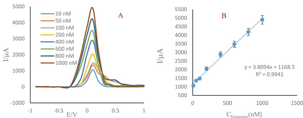
Fig. 6 (A) SWVs of the engineered sensor in different concentrations of histamine biomarker (10, 50, 100, 200, 400, 600, 800 and 1000 nM). (B) Relationship between  $I_{pa}$  and histamine concentration in meat sample.  $T_{eq} = 2$ ,  $E_{being} = -1$  V,  $E_{end} = 1$  V,  $E_{step} = 0.1$  V, amplitude = 0.001 V, frequency = 10 Hz using  $K_3[Fe(CN)_6]/K_4[Fe(CN)_6]$  (5 mM) as the supporting electrolyte.
