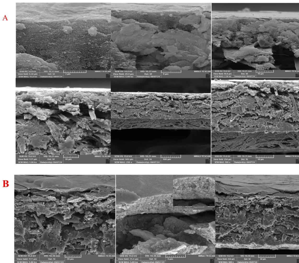
Fig. 3 Cross FE-SEM images of microelectrode prepared by conductive nano-silver ink before (A), after incubation with histamine (B) at various magnifications.
