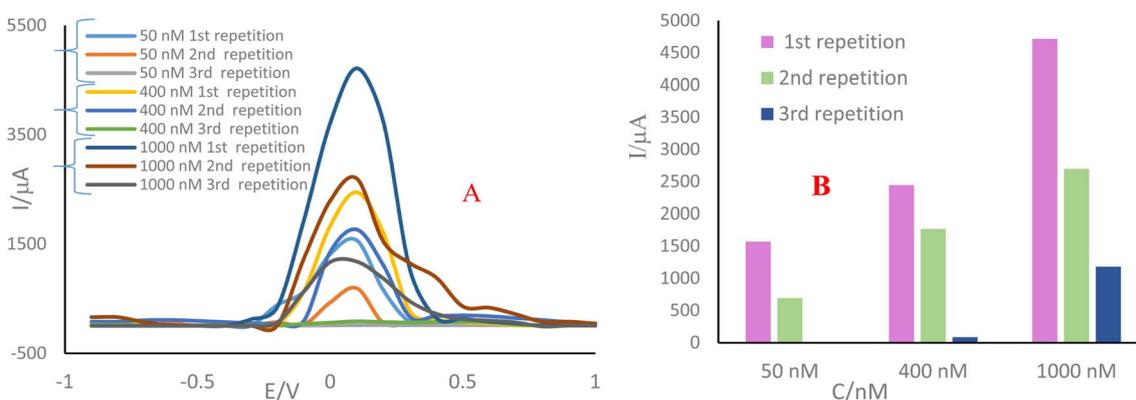
Fig. 8 (A) Three consecutive SWVs of the three microscale sensor drop cast by various concentrations of histamine (50, 400, and 1000 nM). The supporting electrolyte was 10 mL of  $K_3[Fe(CN)_6]/K_4[Fe(CN)_6]$  (5 mM) solution, potential range:  $-1$  to  $1$  V, Sweep rate =  $100$   $mV s^{-1}$ . (B) Corresponding histogram.
