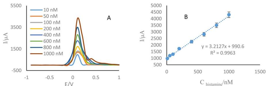
Fig. 5 (A) SWVs of the engineered sensor (Ag ink/Ag ink) in different concentrations of histamine (10, 50, 100, 200, 400, 600, 800, 1000 nM). (B) Relationship between  $I_{pa}$  and histamine concentration in standard sample.  $t_{eq} = 2$ ,  $E_{being} = -1$  V,  $E_{end} = 1$  V,  $E_{step} = 0.1$  V, amplitude = 0.001 V, frequency = 10 Hz using  $K_3[Fe(CN)_6]/K_4[Fe(CN)_6]$  (5 mM) as the supporting electrolyte.
