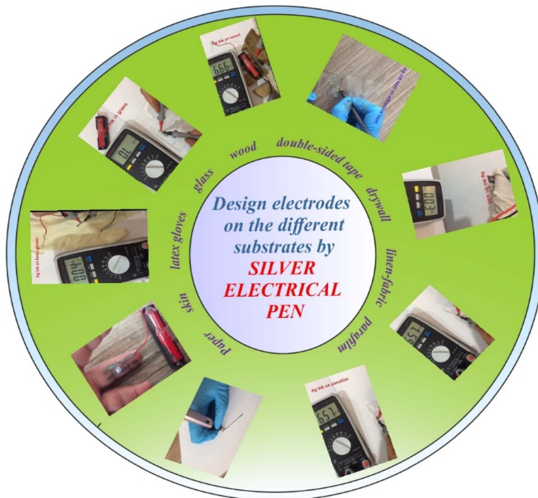
Scheme 3 Design electrodes on the different substrates by silver electrical pen.
