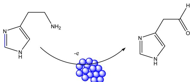
Scheme 5 Detection mechanism of histamine using conductive nano-silver ink paper-based sensor.
