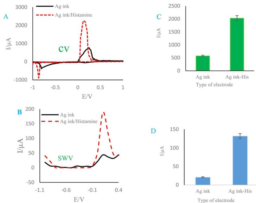
Fig. 1 (A and B) CVs and SWVs of paper modified conductive nano-silver ink and Ag ink/histamine in the presence of  $\text{K}_3[\text{Fe}(\text{CN})_6]/\text{K}_4[\text{Fe}(\text{CN})_6]$  (5 mM) at the potential range of  $-1$  to  $+1$  V and sweep rate of  $100 \text{ mV s}^{-1}$ , respectively. (C and D) Histograms of peak current versus type of electrode obtained from CVs, SWVs respectively. (E) EIS of paper modified conductive nano-silver ink and Ag ink/histamine.
