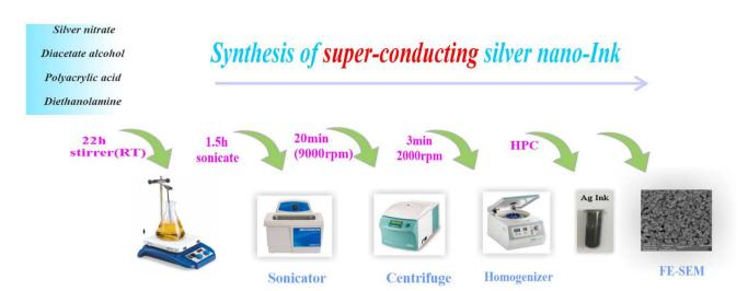
Scheme 2 Super-conductive Ag-nanoink preparation procedure.
