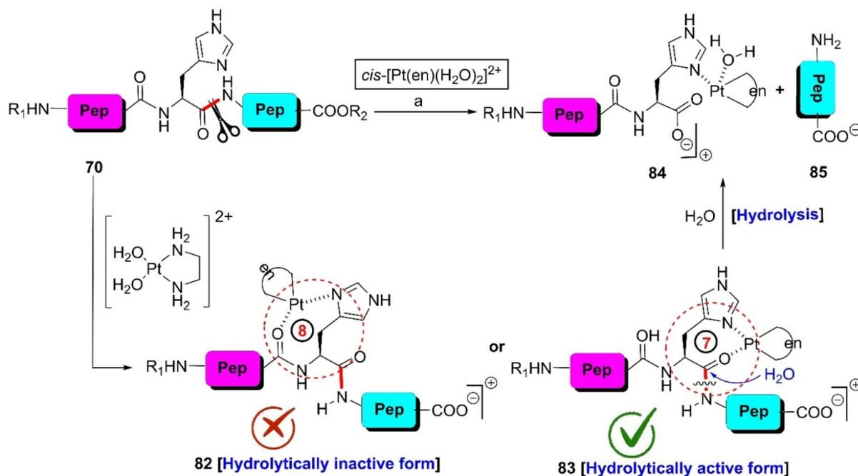
Scheme 13 H-selective cleavage of peptide bonds via metal complexation. Reaction conditions: (a) peptide : Pt(II)-complex = 1 : 1 or 1 : 2, H<sub>2</sub>O, pH 2.65, 60 °C.
