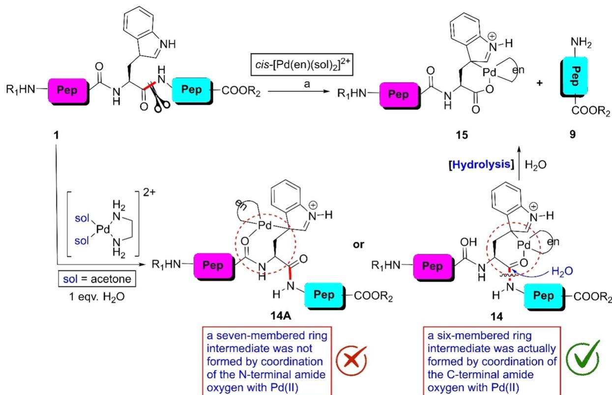
**Scheme 1** W-selective scissoring of peptides through metal complexation. Reaction conditions: (a) peptide : metal complex = 1 : 1, acetone-*d*<sub>6</sub>, DCIO<sub>4</sub>, 50 °C. (This experiment was performed in an NMR tube).
