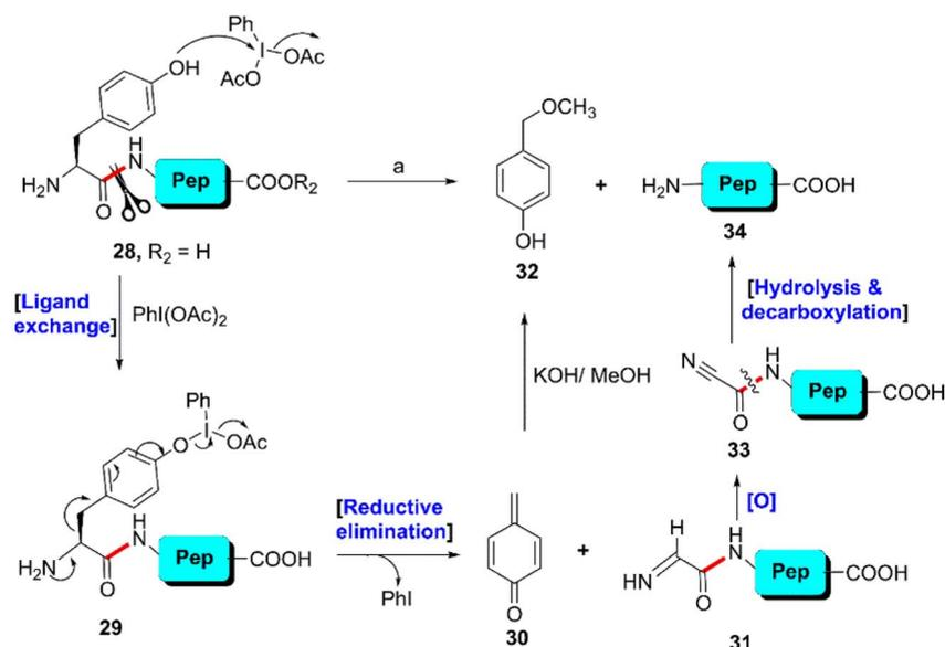
**Scheme 5** Y-selective cleavage of the peptide bond through oxidation using hypervalent iodine. Reaction conditions: (a) PhI(OAc)<sub>2</sub>, KOH–MeOH, 0–5 °C, 1.5 h, 60–80%.
