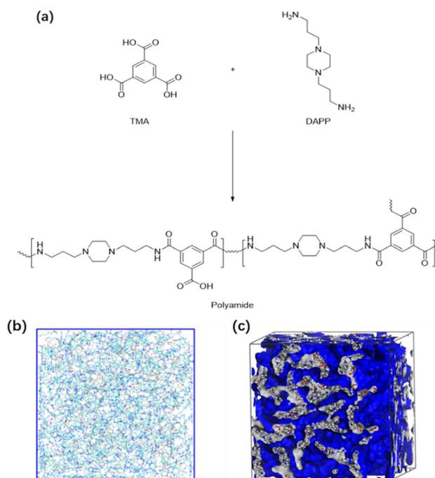
Fig. 5 (a) Structure formula of DAPP and TMA monomers and the crosslinked polyamide. (b) Snapshot of the initial system. (c) 3D pore size distribution map. The box size is  $6.0 \times 6.0 \times 6.0 \text{ nm}^3$  and the density is  $0.8 \text{ g cm}^{-3}$ .
