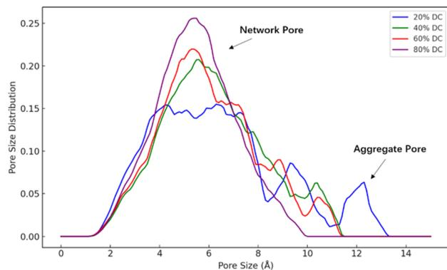
**Fig. 8** PSD of the solvated membranes formed by DAPP and TMA with different DC. Aggregate pores are larger pores formed by loose packing or incompletely cross-linked regions between polymer chains. Network pores are small, uniform pores formed by a highly cross-linked network of polymer chains.
