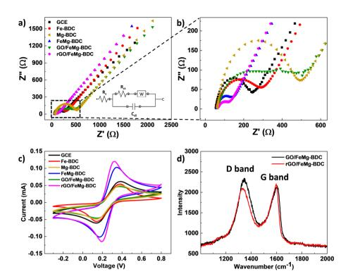
Fig. 4 (a and b) Nyquist plots and (c) CV redox current response at a scan rate of  $0.05 \text{ V s}^{-1}$  of the prepared electrodes in 0.1 M KCl solution containing 5 mM of [Fe(CN)<sub>6</sub>]<sup>3-/4-</sup>, (d) Raman spectrum of GO/FeMg-BDC and rGO/FeMg-BDC.
