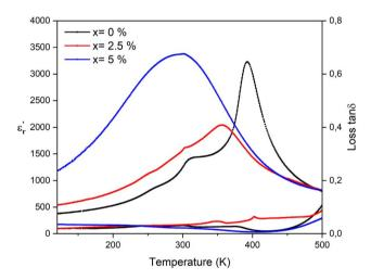
Fig. 3 Temperature dependence of the real part of the dielectric constant  $(\varepsilon_r')$  and the dielectric loss  $(\tan\delta)$  for BCTZ-xZN ceramics.
