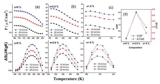
Fig. 6 (a–c) Polarization change ( $\Delta P$ ) and entropy change ( $\Delta S$ ) in BCTZ-xZN ceramics. (d) Maximum value of the coefficient of performance (COP) and electrocaloric responsivity ( $\Delta T/\Delta E$ ) for BCTZ-xZN ceramics.
