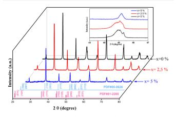
Fig. 1 X-ray diffraction (XRD) patterns of BCTZ-xZN ceramics. The inset shows the peak located at 45°.
