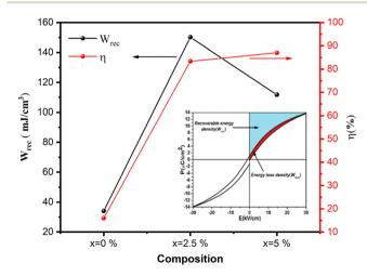
Fig. 5 Variation of the recoverable energy density ( $W_{rec}$ ) (black) and energy storage efficiency  $(\eta)$ (red). The inset method for calculating energy storage efficiency from P-E loops.
