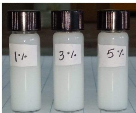
Fig. 10 Colloidal stability of final latex containing different amounts of MMT-ADM 18 over 3 months.
