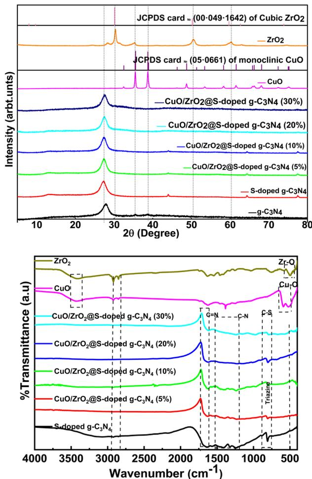
Fig. 2 XRD pattern (top) and FT-IR (bottom) of  $g\text{-C}_3\text{N}_4$  and S-doped  $g\text{-C}_3\text{N}_4$ ,  $\text{CuO/ZrO}_2@S\text{-doped } g\text{-C}_3\text{N}_4$  (5, 10, 20, and 30%) NCs, pure CuO and pure  $\text{ZrO}_2$  NPs.
