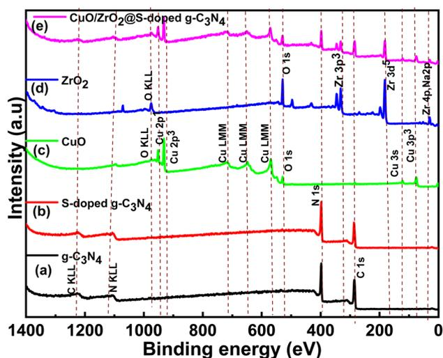
Fig. 9 X-ray photoelectron survey spectra for (a) g-C<sub>3</sub>N<sub>4</sub>, (b) S-doped g-C<sub>3</sub>N<sub>4</sub>, (c) CuO, (d) ZrO<sub>2</sub> and (e) CuO/ZrO<sub>2</sub>@S-doped g-C<sub>3</sub>N<sub>4</sub> NCs.
