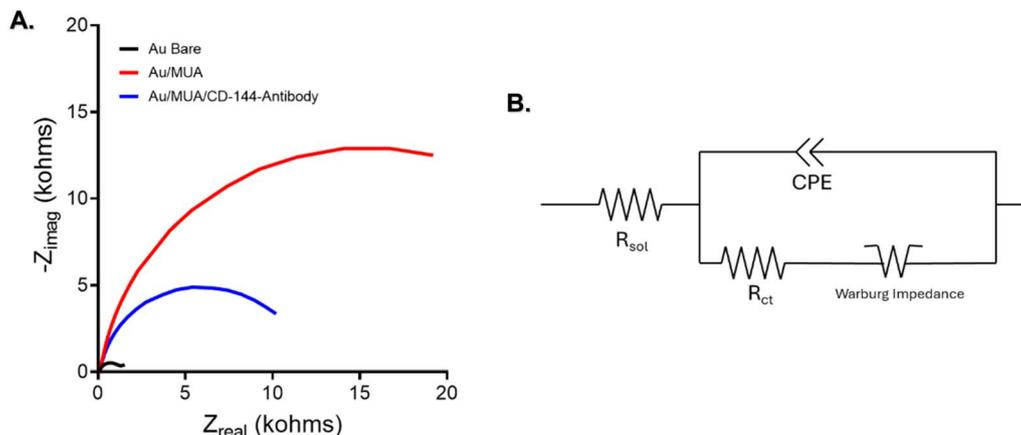
**Fig. 4** (A) EIS Nyquist plot of functionalization of the Au-SPE with MUA and Cd-144 antibody. (B) A model of CPE with diffusion was used in the simulation to calculate the electron-transfer resistance.
