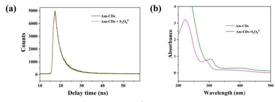
Fig. 4 (a) Fluorescence decay curve of Am-CDs without and with  $S_2O_8^{2-}$ . (b) UV-vis absorption spectra of Am-CDs without and with  $S_2O_8^{2-}$ .
