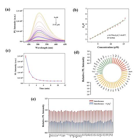
Fig. 3 (a) Fluorescence quenching of Am-CDs in the presence of  $S_2O_8^{2-}$  (0–27.91  $\mu$ M). (b) Linear relationship between  $F_0/F$  and  $S_2O_8^{2-}$  concentration (1.96–15.59  $\mu$ M). (c) Reaction time of the system. (d and e) Selectivity and anti-interference patterns of the system, respectively.
