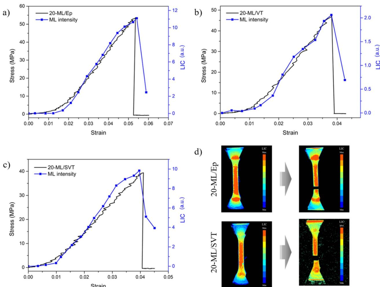
Fig. 4 ML intensity of (a) ML/EP, (b) ML/VT and (c) ML/SVT under single static loading with a strain rate of  $100 \mu\text{m s}^{-1}$  (d) binarized and colored images of ML-epoxy samples before and after fracture.
