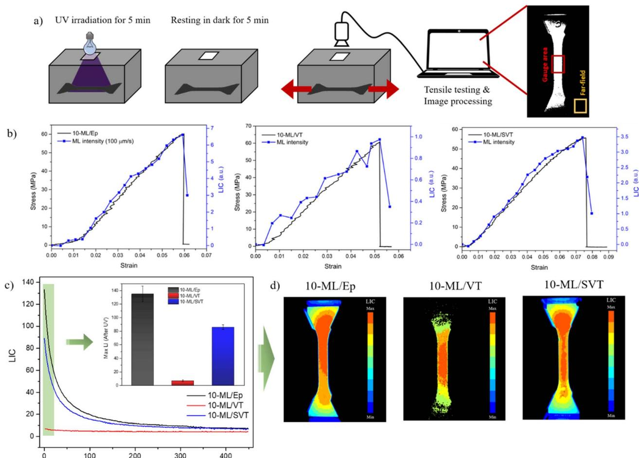
Fig. 3 (a) Schematic overview of ML intensity test set-up in dark environment (b) light intensity change (LIC) of ML-epoxy sensors under single static loading with a strain rate of  $100 \mu\text{m s}^{-1}$  (c) afterglow intensity change of commercial epoxy and epoxy vitrimers under same excitation conditions (inset: maximum light intensity after 5 minutes of UV-excitation) (d) visualization of maximum light intensity variation in ML/Ep, ML/VT and ML/SVT after UV excitation.
