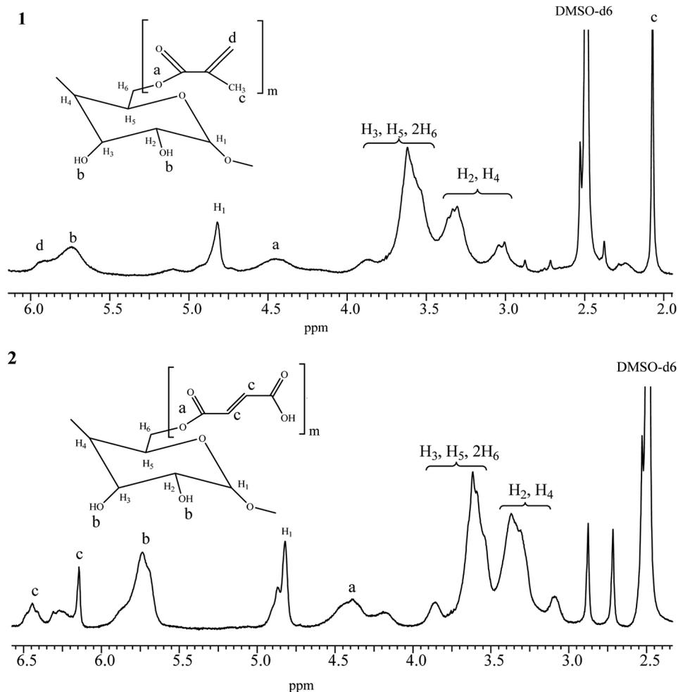
Fig. 2  $^1\text{H}$  NMR spectra of  $\beta$ -cyclodextrin derivatives: (1) –  $\beta$ -CD methacrylate ( $m = 5$ ), (2) –  $\beta$ -CD maleate ( $m = 5$ ).
