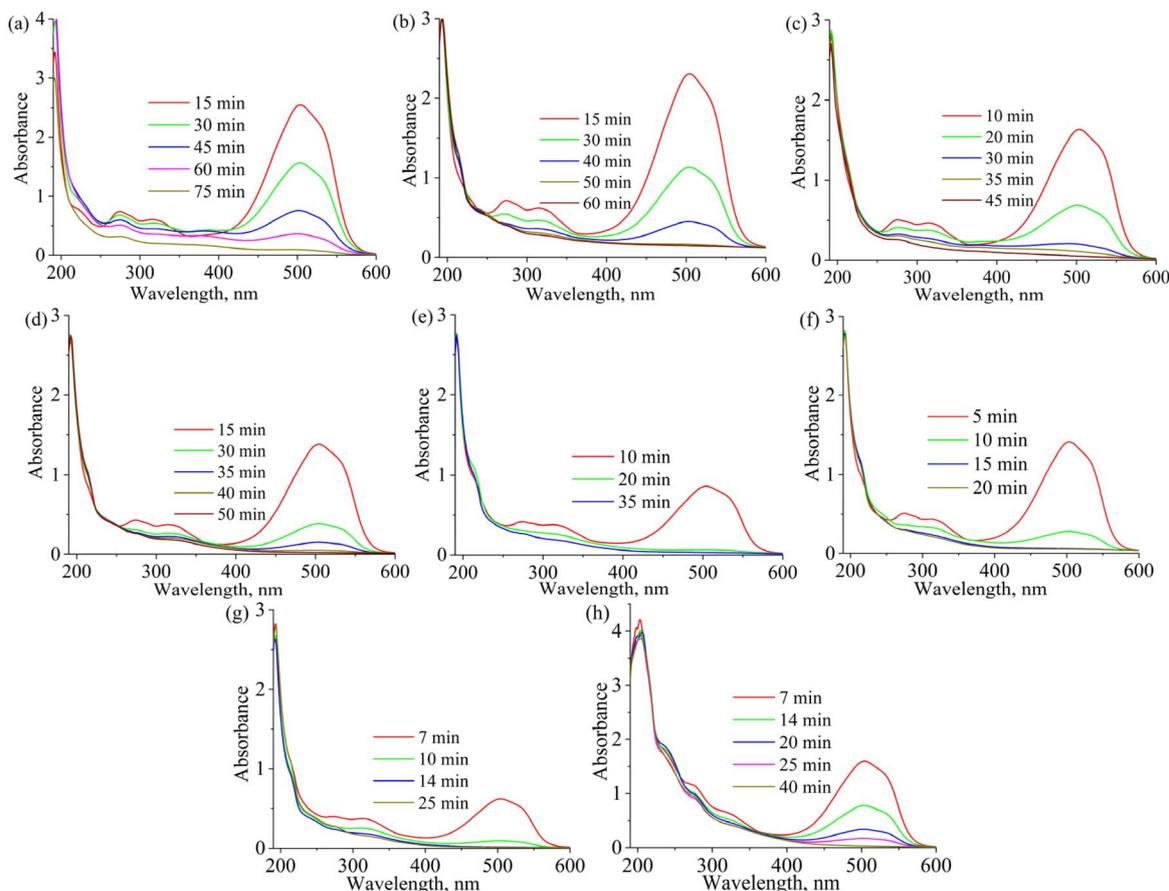
Fig. 10 UV-vis spectra of MO solutions after irradiation using  $TiO_2$  (a),  $TiO_2$ -P3 (b),  $TiO_2$ /Ag<sub>7</sub>CD/CD (c),  $TiO_2$ -P10 (d),  $TiO_2$ -P11Ag (e),  $TiO_2$ -P13Ag (f),  $TiO_2$ -P15Ag 1st cycle (g), and  $TiO_2$ -P15Ag 5th cycle (h).
