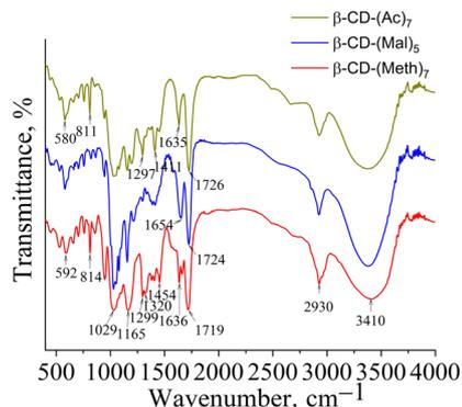
Fig. 3 FTIR spectra of  $\beta$ -CD monomers.
