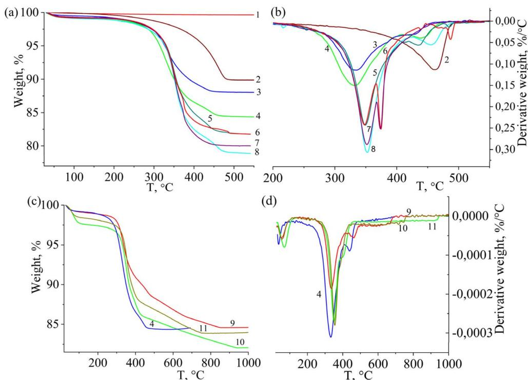
Fig. 8 TGA (a and c) and DTG (b and d) curves of TiO<sub>2</sub> (1), TiO<sub>2</sub>-P1 (2), TiO<sub>2</sub>-P8Ag (3), TiO<sub>2</sub>-P3 (4), TiO<sub>2</sub>-P13Ag (5), TiO<sub>2</sub>-P11Ag (6), TiO<sub>2</sub>-P10Ag (7), TiO<sub>2</sub>-P10 (8), TiO<sub>2</sub>-P3\* (9), TiO<sub>2</sub>-P14\* (10), and TiO<sub>2</sub>-P15-Ag\* (11).
