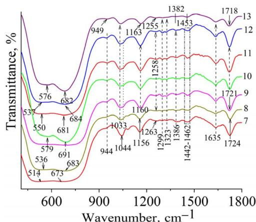
Fig. 5 FTIR spectra of TiO<sub>2</sub>-P5Ag (7), TiO<sub>2</sub>-P8Ag (8), TiO<sub>2</sub>-P11Ag (9), TiO<sub>2</sub>-P10Ag (10), TiO<sub>2</sub>-P12Ag (11), TiO<sub>2</sub>-P13Ag (12), and TiO<sub>2</sub>-P15Ag (13).
