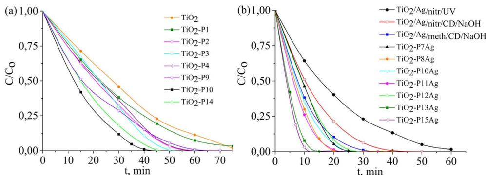
Fig. 9 Photocatalytic degradation curves of methyl orange with  $TiO_2$ ,  $TiO_2$ /CDP,  $TiO_2$ /AgNPs, and  $TiO_2$ /CDP/AgNPs (conditions:  $C_0$  (MO) = 25 mg L<sup>-1</sup>,  $V$  = 80 ml, and pH 2.5).
