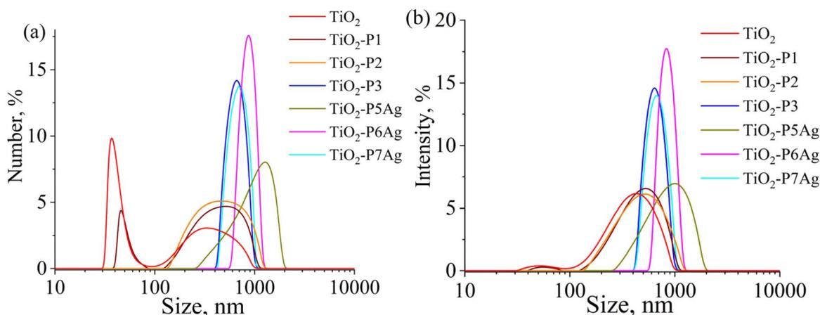
Fig. 6 Particle size distributions by number (a) and intensity (b) of TiO<sub>2</sub> and TiO<sub>2</sub>/CD copolymers.
