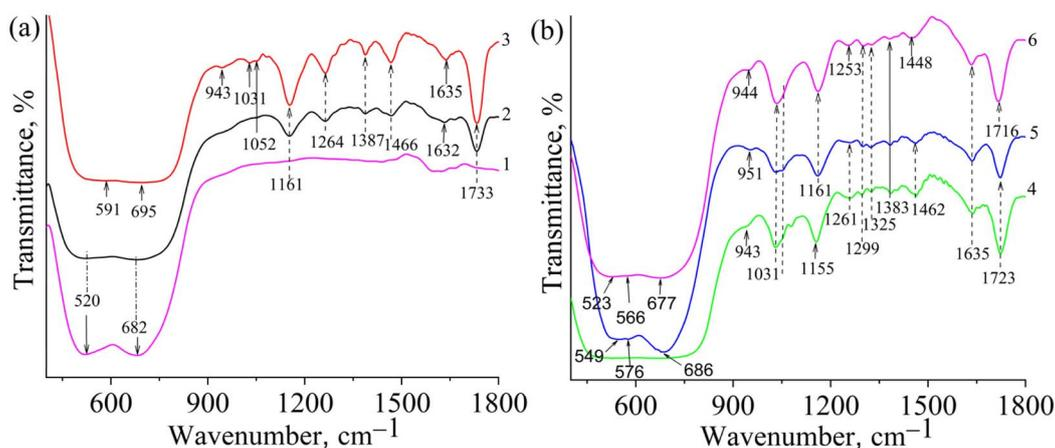
Fig. 4 FTIR spectra of  $\text{TiO}_2$  (1),  $\text{TiO}_2\text{-P1}$  (2),  $\text{TiO}_2\text{-P2}$  (3),  $\text{TiO}_2\text{-P3}$  (4),  $\text{TiO}_2\text{-P10}$  (5) and  $\text{TiO}_2\text{-P14}$  (6).
