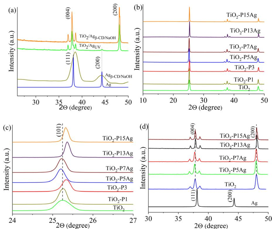
Fig. 7 XRD patterns of TiO<sub>2</sub>, TiO<sub>2</sub>/AgNPs (a), TiO<sub>2</sub>/CDP (b), and TiO<sub>2</sub>/CDP/AgNPs (c and d – enlarged b).
