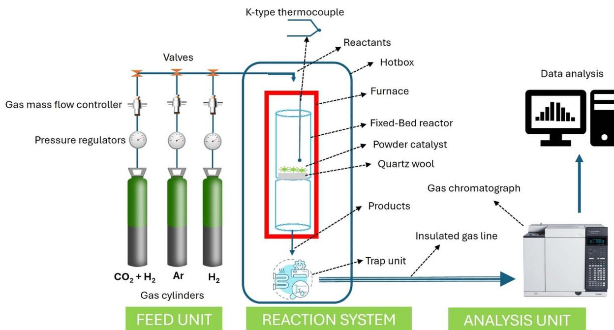
Fig. 1 Experimental setup for the CO<sub>2</sub> methanation reaction.
