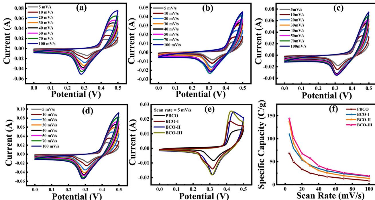
Fig. 5 CV curves at different scan rates for (a) PBCO, (b) BCO-I, (c) BCO-II, (d) BCO-III, and (e) comparison of all samples at 5 mV s<sup>-1</sup>, and (f) scan rate vs. specific capacity.
