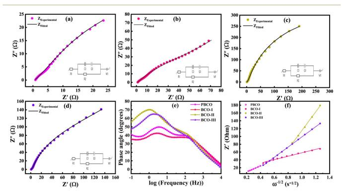
Fig. 10 (a–d) EIS circuit fitting spectra for PBCO, BCO-I, BCO-II, and BCO-III, respectively, (e) Bode plot for all the prepared samples (f) Warburg coefficients from linear fitting between  $\omega^{-1/2}$  vs. real part of impedance for all the prepared samples.
