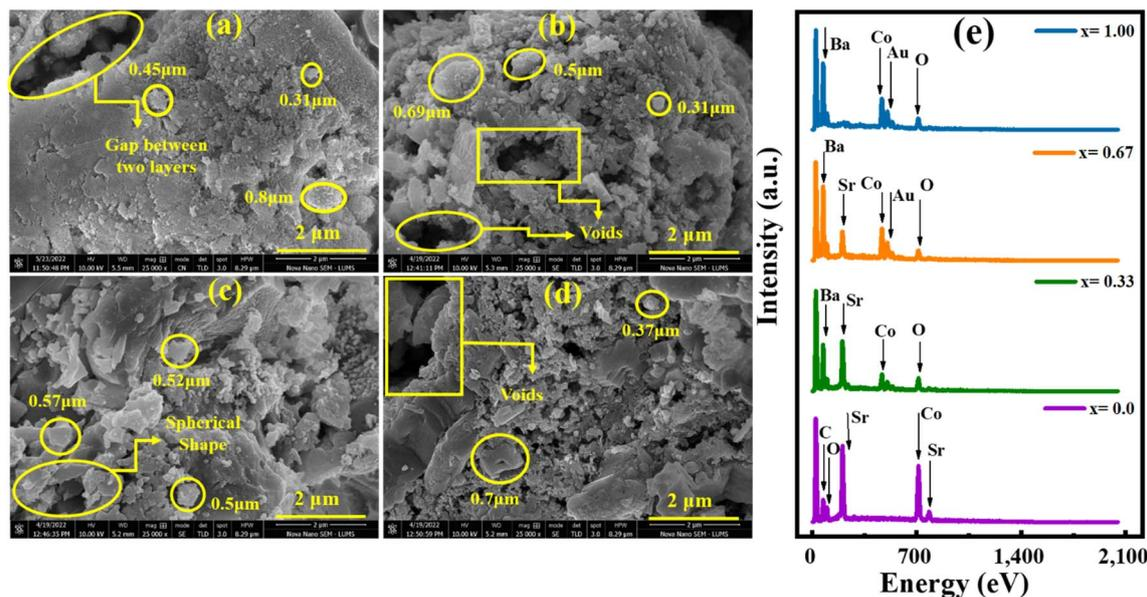
Fig. 3 (a–d) FESEM images of  $\text{Sr}_{1-x}\text{Ba}_x\text{CoO}_3$  ( $x = 0.00, 0.33, 0.67, \text{ and } 1.00$ ) and (e) EDX spectra of  $\text{Sr}_{1-x}\text{Ba}_x\text{CoO}_3$  ( $x = 0.00, 0.33, 0.67, \text{ and } 1.00$ ).
