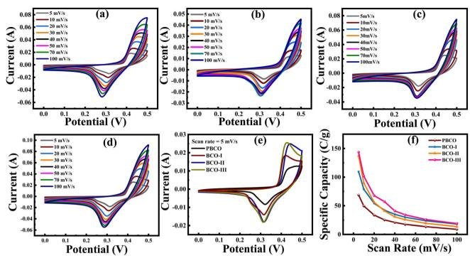
Fig. 5 CV curves at different scan rates for (a) PBCO, (b) BCO-I, (c) BCO-II, (d) BCO-III, and (e) comparison of all samples at 5 mV s<sup>-1</sup>, and (f) scan rate vs. specific capacity.
