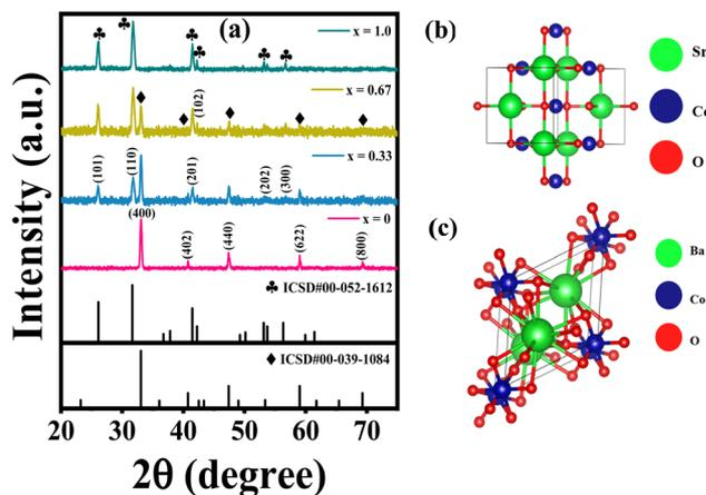
Fig. 2 (a) Standard diffraction and XRD patterns of Sr<sub>1-x</sub>Ba<sub>x</sub>CoO<sub>3</sub> and (b and c) crystal structures of SrCoO<sub>3</sub> and BaCoO<sub>3</sub>.
