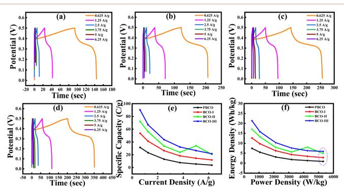
Fig. 8 GCD curves at different current densities for (a) PBCO, (b) BCO-I, (c) BCO-II, (d) BCO-III, and (e) current density vs. specific capacity, and (f) power density vs. energy density.
