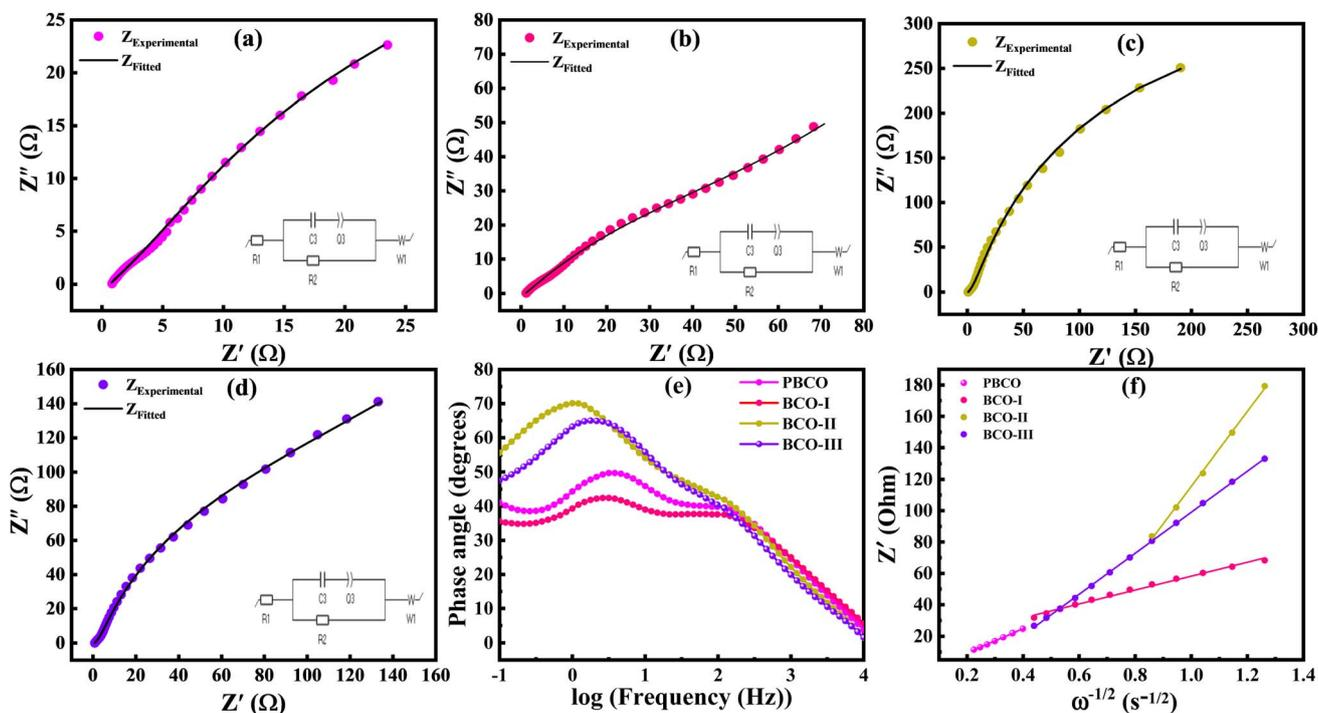
Fig. 10 (a–d) EIS circuit fitting spectra for PBCO, BCO-I, BCO-II, and BCO-III, respectively, (e) Bode plot for all the prepared samples (f) Warburg coefficients from linear fitting between  $\omega^{-1/2}$  vs. real part of impedance for all the prepared samples.
