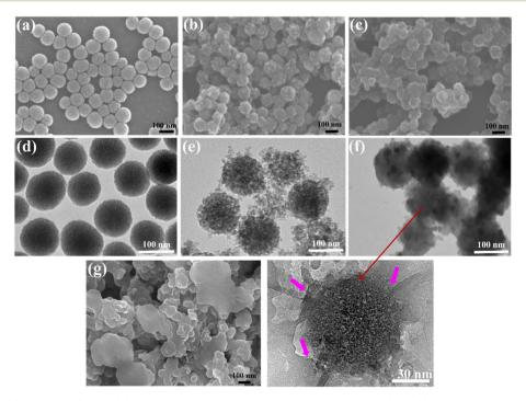
Fig. 3 SEM images of (a) silica NPs, (b) PSi, (c) IPSi-Di-DQA, and TEM images of (d) silica NPs, (e) PSi, (f) IPSi-Di-DQA, (g) IPSi-Di-DQA after NIR irradiation and drug release.
