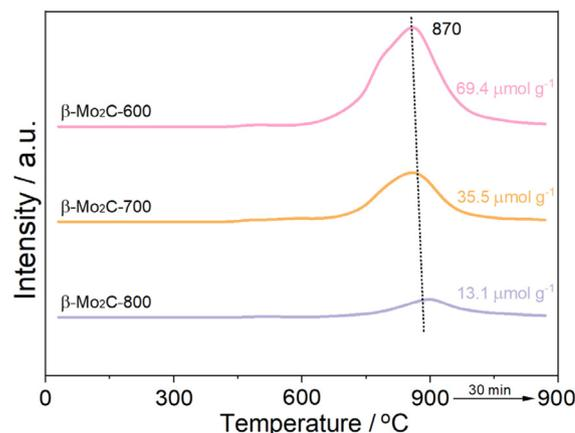
Fig. 6 CO-TPD curves of β-Mo<sub>2</sub>C-600, β-Mo<sub>2</sub>C-700, and β-Mo<sub>2</sub>C-800 catalysts.
