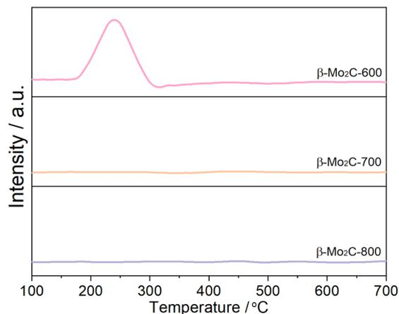
Fig. 3 H<sub>2</sub>-TPR profiles of non-passivated  $\beta$ -Mo<sub>2</sub>C-600,  $\beta$ -Mo<sub>2</sub>C-700, and  $\beta$ -Mo<sub>2</sub>C-800 catalysts. The non-passivated samples were directly subjected to H<sub>2</sub>-TPR experiment, where they were heated from 100 to 700 °C at a rate of 5 °C min<sup>-1</sup> in a gas mixture of 5%H<sub>2</sub>/Ar (60 ml min<sup>-1</sup>).
