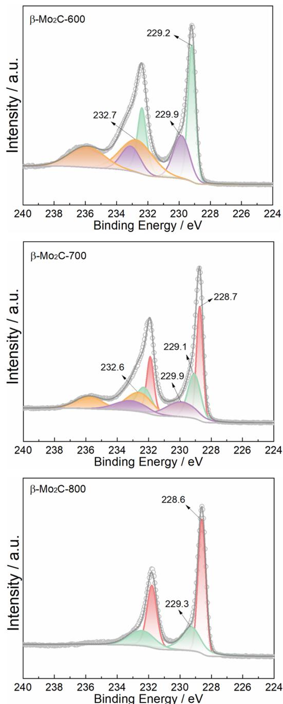
Fig. 4 XPS spectra of Mo 3d region of  $\beta$ -Mo<sub>2</sub>C-600,  $\beta$ -Mo<sub>2</sub>C-700, and  $\beta$ -Mo<sub>2</sub>C-800 catalysts.
