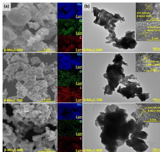
Fig. 2 (a) SEM images and (b) TEM images of  $\beta$ -Mo<sub>2</sub>C-600,  $\beta$ -Mo<sub>2</sub>C-700, and  $\beta$ -Mo<sub>2</sub>C-800 catalysts. The insets in the SEM images show the Mo, O and C element mapping images and those in the TEM images show the  $\beta$ -Mo<sub>2</sub>C (002) and MoOC (111) crystal lattices.
