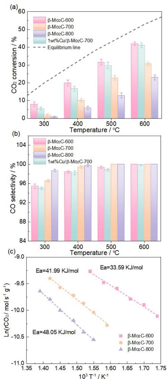
Fig. 5 (a) CO<sub>2</sub> conversion and (b) CO selectivity over β-Mo<sub>2</sub>C-600, β-Mo<sub>2</sub>C-700, and β-Mo<sub>2</sub>C-800 catalysts in the RWGS reaction as well as 1 wt% Cu/β-Mo<sub>2</sub>C-700 catalyst for comparison (reaction conditions: CO<sub>2</sub>/H<sub>2</sub> = 1/2, WHSV = 150 000 cm<sup>3</sup> g<sup>-1</sup> h<sup>-1</sup>, T = 300–600 °C) and (c) Arrhenius plots and E<sub>a</sub> values below 15% of CO<sub>2</sub> conversion.
