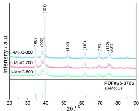
Fig. 1 XRD patterns of the  $\beta$ -Mo<sub>2</sub>C catalysts obtained at different carbonization temperatures of 600, 700 and 800 °C.
