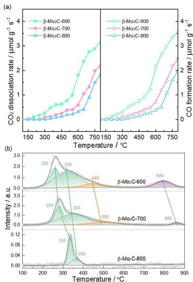
Fig. 7 (a) CO<sub>2</sub>-TPO and (b) H<sub>2</sub>-TPR profiles of passivated β-Mo<sub>2</sub>C-600, β-Mo<sub>2</sub>C-700, and β-Mo<sub>2</sub>C-800 catalysts.
