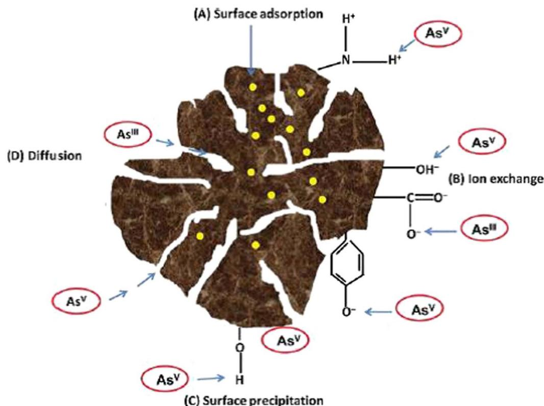
Fig. 4 Illustration of the mechanism of arsenic sorption on the surface of a biosorbent.<sup>152</sup>
