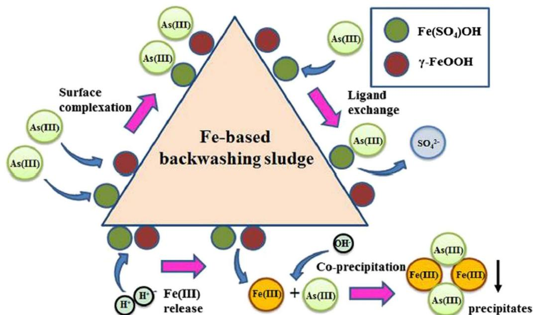
Fig. 3 Suggested mechanisms for removing As<sup>III</sup> using FBBS as an adsorbent, with permission from Wu *et al.* 2013.<sup>151</sup>
