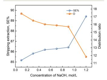
Fig. 14 The relationship between the concentration of stripping agent and stripping rate and distribution ratio.
