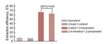
Fig. 3 Effect of different extractants on extraction rate.
