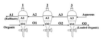
Fig. 2 Flow chart of three-stage continuous countercurrent extraction.
