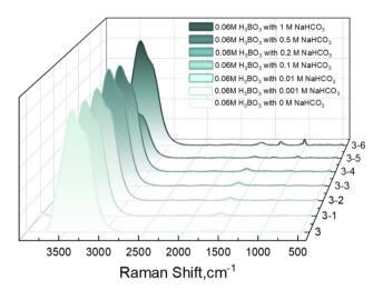
Fig. 17 Raman spectra of boric acid with fixed concentration and sodium bicarbonate with different concentration.
