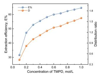
Fig. 5 Effect of TMPD concentration on boron extraction.
