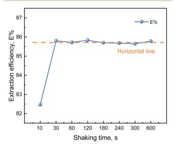
Fig. 8 The relationship between mixing time and extraction rate.
