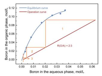
Fig. 20 Boron extraction distribution isotherm and McCable-Thiele diagram.
