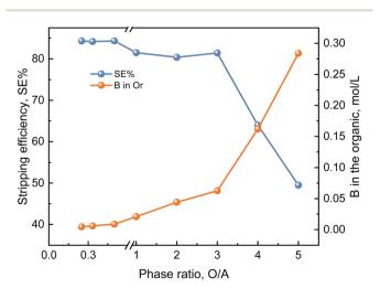
Fig. 15 Compared to the effect on stripping efficiency.
