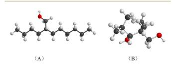
Fig. 1 Molecular structure diagram, (A) is 2-butyl-1-octanol, (B) is TMPD.
