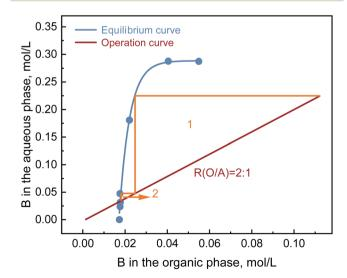
Fig. 21 Boron stripping extraction distribution isotherm and McCable-Thiele diagram.
