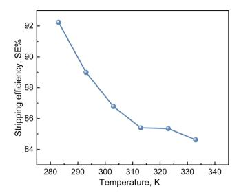
Fig. 16 Effect of temperature on stripping efficiency.
