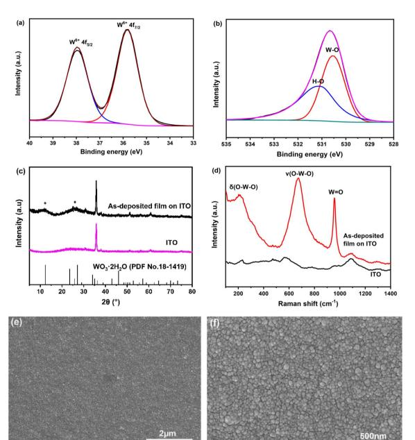
Fig. 2 Structural and morphological characterization of the amorphous  $WO_3 \cdot 2H_2O$  film electrodeposited on the ITO substrate: (a) and (b) high-resolution W4f and O1s XPS spectra, (c) XRD pattern, (d) Raman spectrum, (e) and (f) SEM images.
