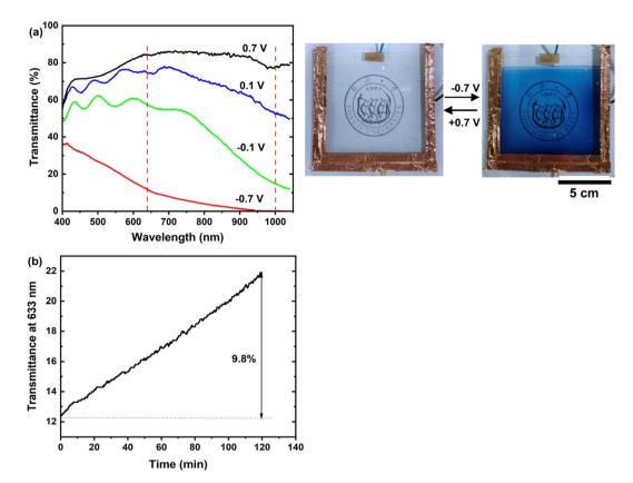
Fig. 6 (a) Optical transmittance of a 10 cm  $\times$  10 cm device at various potentials, along with photographs of the device in its bleached state at 0.7 V and colored state at -0.7 V; (b) evolution of transmittance at 633 nm under open circuit voltage (OCV) after coloration at -0.7 V.
