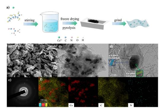
Fig. 1 (a) Schematic of the synthesis of  $V_0$ –CeO<sub>2</sub>/C-1300. (b) SEM image, (c–e) TEM image, and (f) EDS elemental mappings of  $V_0$ –CeO<sub>2</sub>/C-1300.
