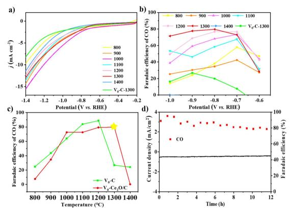
Fig. 4 (a and b) LSV curves and  $FE_{CO}$  of  $V_0$ – $CeO_2/C$  at different temperatures and  $V_0$ –C-1300. (c)  $FE_{CO}$  of  $V_0$ – $CeO_2/C$  and  $V_0$ –C at different temperatures. (d) Stability test at -0.80 V of  $V_0$ – $CeO_2/C$ -1300.
