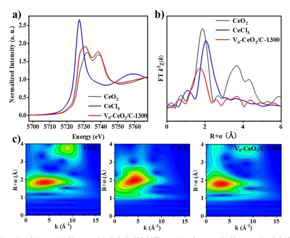
Fig. 3 (a) Normalized Ce  $L_3$ -edge XANES spectra of  $V_0$ -CeO<sub>2</sub>/C-1300, (b) FT  $k_3$ -weighted Ce  $L_3$ -edge EXAFS spectra of  $V_0$ -CeO<sub>2</sub>/C-1300 and the references, and (c) wavelet transform EXAFS of V<sub>0</sub>-CeO<sub>2</sub>/C-1300.
