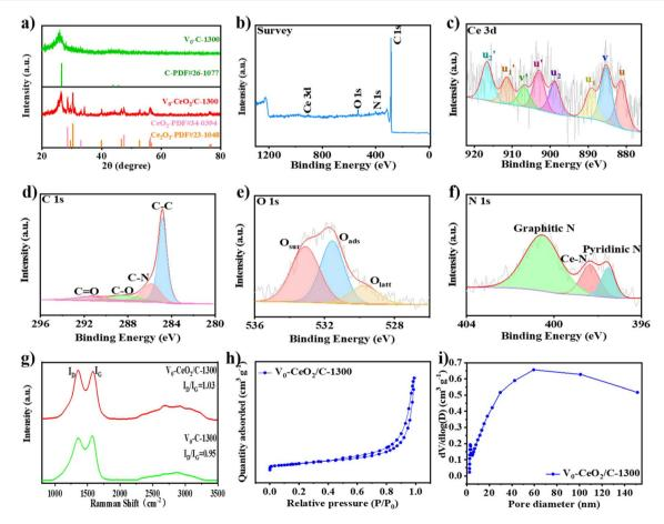
Fig. 2 (a) XRD patterns. XPS spectra of  $V_0$ —CeO<sub>2</sub>/C-1300: (b) survey spectrum, (c) Ce 3d spectrum, (d) C 1s spectrum, (e) O 1s spectrum and (f) N 1s spectrum. (g) Raman spectrum, (h)  $N_2$  adsorption/desorption isotherms and (i) pore size distribution.
