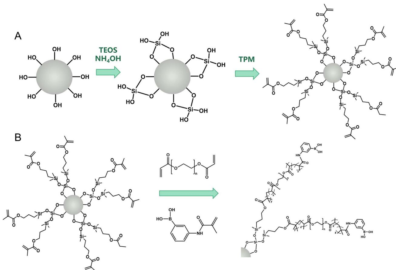
Fig. 1 Schematic illustration of the synthesis method of  $\text{Fe}_3\text{O}_4$ @poly(PEGDA-co-MAAPBA) NPs. The phenylboronic acid-functionalized  $\text{Fe}_3\text{O}_4$  NPs were prepared through a two-step strategy: (A) the preparation of double-bond functionalized  $\text{Fe}_3\text{O}_4$  NPs, and (B) the copolymerization of double-bond functionalized  $\text{Fe}_3\text{O}_4$  NPs, cross-linker PEGDA, and functional monomer MAAPBA.
