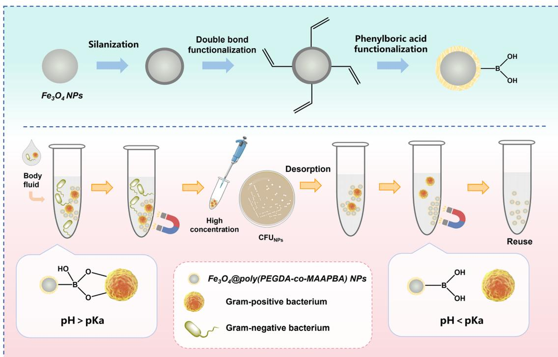
**Scheme 1** Schematic illustration of the synthesis steps of the phenylboronic acid-functionalized  $\text{Fe}_3\text{O}_4$  nanoparticles ( $\text{Fe}_3\text{O}_4$ @poly(PEGDA-co-MAAPBA) NPs), and the applications in enriching and diagnosing low abundances of pathogenic bacteria.
