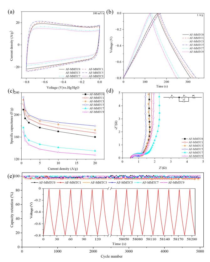
Fig. 4 Electrochemical properties of heteroatom-doped hierarchical porous carbon in three-electrode system. (a) CV curves, (b) GCD curves, (c) specific capacitance at different current densities, (d) EIS curves and (e) cycling stability (inset plots show the front-end and back-end charging/discharging curves of the AF-MMTC5 samples during a long cycling process).
