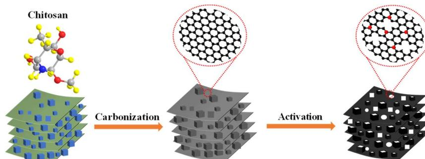
Fig. 1 Schematic diagram of the preparation process of heteroatom-doped hierarchical porous carbon.
