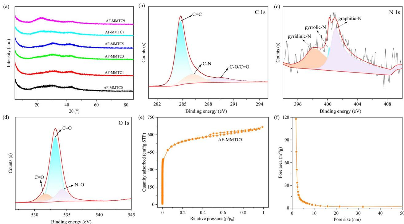
Fig. 3 (a) The XRD patterns of AF-MMTCs, (b) C 1s, (c) N 1s, (d) O 1s, (e) N<sub>2</sub> adsorption–desorption isotherms and (f) pore size distribution of AF-MMTC5.
