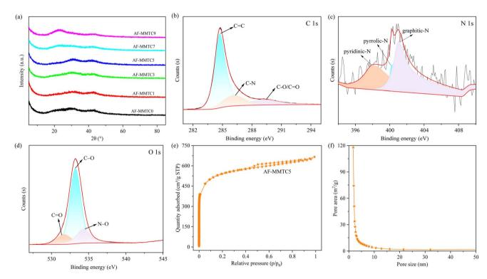
Fig. 3 (a) The XRD patterns of AF-MMTCs, (b) C 1s, (c) N 1s, (d) O 1s, (e)  $N_2$  adsorption—desorption isotherms and (f) pore size distribution of AF-MMTC5.
