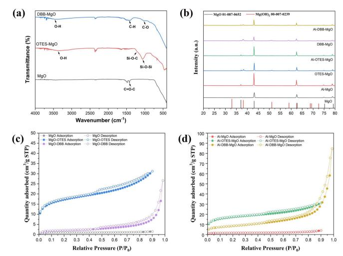
Fig. 2 (a) FTIR spectra of MgO and modified MgO supports; (b) XRD patterns of supports and corresponding catalysts with JCPDS standard cards: 01-087-0652 (MgO) and 00-007-0239 [Mg(OH)<sub>2</sub>]; N<sub>2</sub> adsorption–desorption isotherms of supports (c) and catalysts (d).
