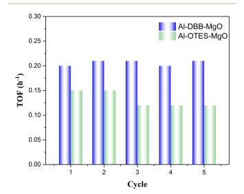
Fig. 5 Recycling performance of modified Al-MgO catalysts (Al-DBB-MgO and Al-OTES-MgO) for the H-transfer reduction of hexanal.
