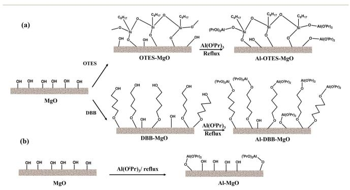
Fig. 1 Processes of (a) MgO support modification followed by Al(O'Pr); immobilization (a); and (b) Al(O'Pr); immobilization onto MgO directly (b).
