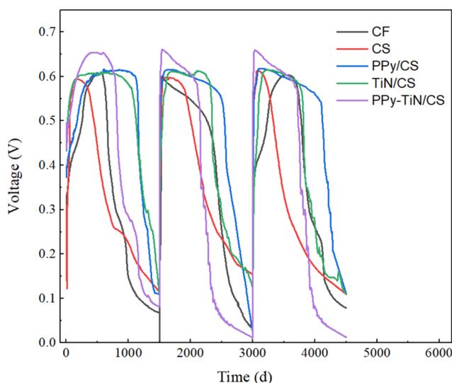
Fig. 9 Output voltage curves for different anodes.
