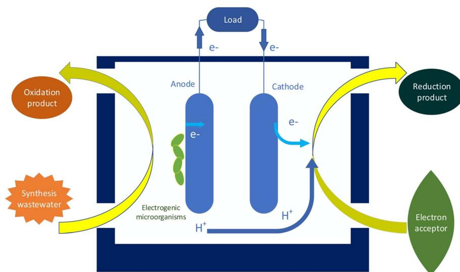
Fig. 1 Schematic diagram of a microbial fuel cell.
