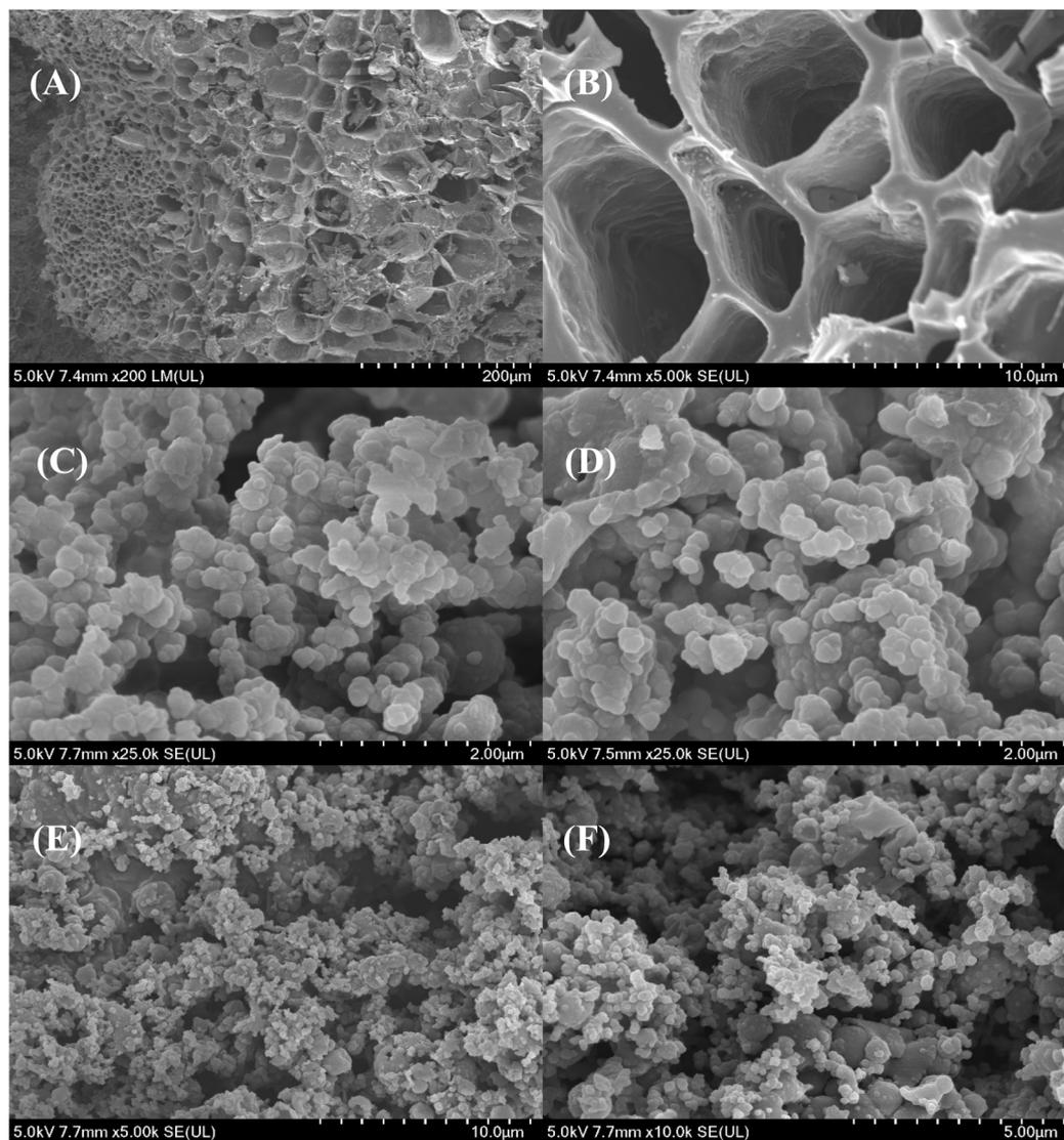
Fig. 3 Scanning electron microscopy analysis of corn straw biochar anode raw materials and modified composite materials (A and B are SEM images of CS biochar materials, C and D are SEM images of PPY/CS modified materials, and E and F are SEM images of PPY-TiN/CS composite modified materials).
