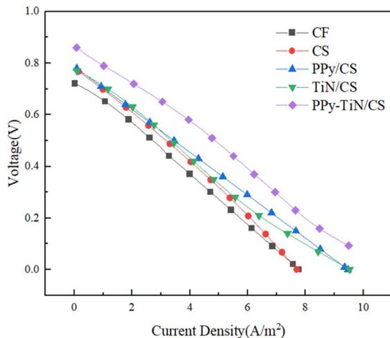
Fig. 11 Polarization curves for different anodes.
