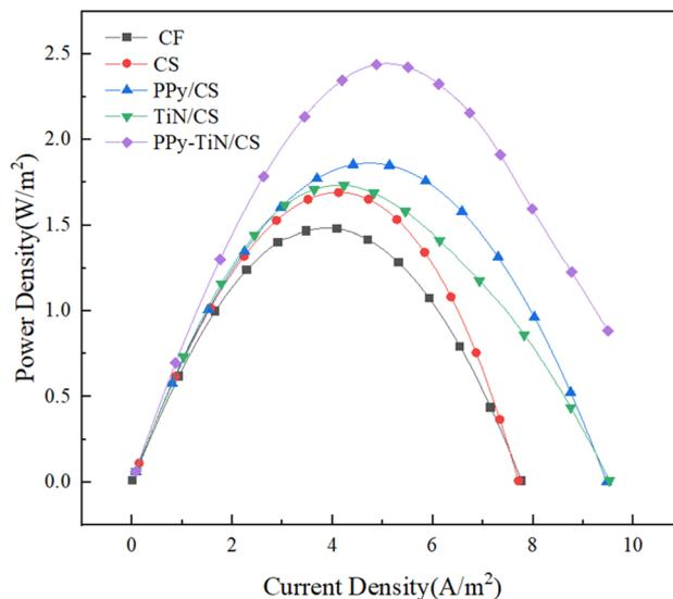
Fig. 10 Power density curves for different anodes.
