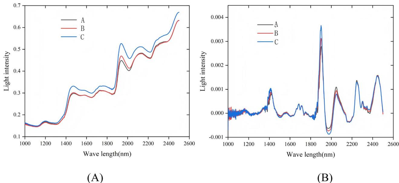
Fig. 2 (A) Averaged absorption spectra for the three moisture levels. (B) 1D spectra for the three moisture levels. In the A, B, and C represent tobacco moisture levels of 5.08%, 12.15%, and 18.09%.
