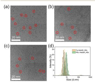
Fig. 1 TEM micrographs of the as-prepared (a) OA-NaGdF<sub>4</sub> NDs, (b) Try-NaGdF<sub>4</sub> NDs and (c) PDL1-NaGdF<sub>4</sub> NDs, and (d) hydrodynamic diameter distribution of Try-NaGdF<sub>4</sub> NDs and PDL1-NaGdF<sub>4</sub> NDs.
