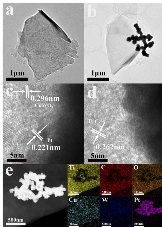
Fig. 1 The TEM images of Ti<sub>3</sub>C<sub>2</sub> (a) and Ti<sub>3</sub>C<sub>2</sub>/CuWO<sub>4</sub>/Pt (b). HRTEM images of Ti<sub>3</sub>C<sub>2</sub>/CuWO<sub>4</sub>/Pt (c) and (d). (e) Elemental mappings for Ti<sub>3</sub>C<sub>2</sub>/CuWO<sub>4</sub>/Pt.
