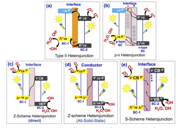
Fig. 7 Various photocatalyst heterojunction interfaces: (a) Type-II heterojunction, (b) P-N heterojunction, (c) direct Z-scheme heterojunction, (d) all-solid-state Z-scheme heterojunction, and (e) S-scheme heterojunction, reprinted with the permission of ref. 121, copyright 2025, Elsevier.
