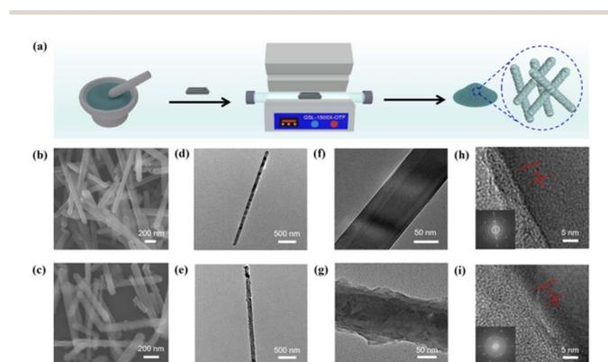
Fig. 1 (a) Schematic representation of the synthesis process for Co-doped  $\text{TiO}_2$  nanorods. Characterization of the synthesized  $\text{TiO}_2$  nanorods: (b) SEM image, (d) TEM image, and (f and h) HRTEM images of pure  $\text{TiO}_2$  nanorods; (c) SEM image, (e) TEM image, and (g and i) HRTEM images of Co-doped  $\text{TiO}_2$  nanorods.
