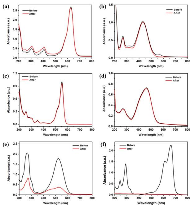
Fig. 3 The UV-Vis absorption curves of different dyes solution before and after adding Co-doped rutile TiO<sub>2</sub> nanorods in the dark at room temperature with 90 min: (a) Brilliant Blue (BB), (b) Cresol Red (CR), (c) Rhodamine B (RhB), (d) Methyl Orange (MO), (e) Neutral Red (NR), (f) Methylene blue (MB) solution.
