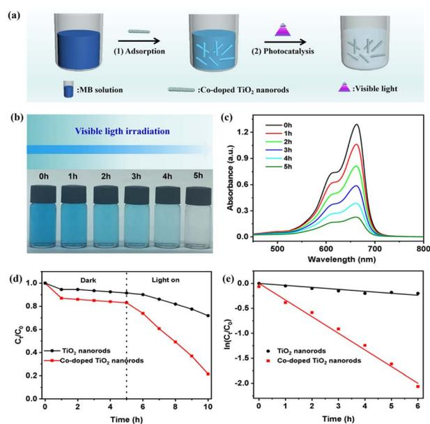
Fig. 4 (a) A schematic representation of the photocatalytic degradation of MB by Co-doped TiO<sub>2</sub> nanorods under visible light, (b) photographs showing the color changes of the MB solution over time, (c) UV-Vis spectra of the degradation of MB during photocatalysis, (d) plots of  $C_t/C_0$  versus time under dark and light conditions, and (e) plots of  $\ln(C_t/C_0)$  versus time for both TiO<sub>2</sub> nanorods and Co-doped TiO<sub>2</sub> nanorods at pH = 7.
