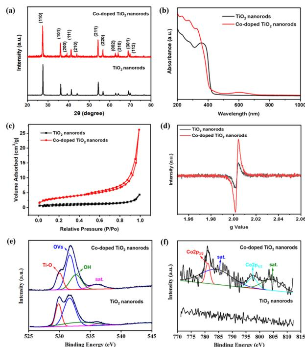
Fig. 2 Characterizations of pure  $\text{TiO}_2$  nanorods and Co-doped  $\text{TiO}_2$  nanorods: (a) XRD pattern, (b) UV-Vis spectra, (c)  $\text{N}_2$  adsorption-desorption isotherms, (d) ESR spectra, (e) O  $1s$  spectra and (f) Co  $2p$  spectra.
