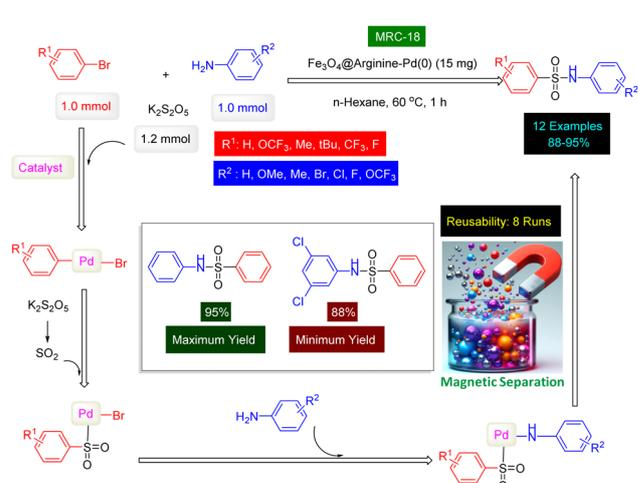
Scheme 18 Fe<sub>3</sub>O<sub>4</sub>@arginine-Pd(0) (MRC-18) catalyzed preparation of *N*-aryl sulfonamides from K<sub>2</sub>S<sub>2</sub>O<sub>8</sub>.
