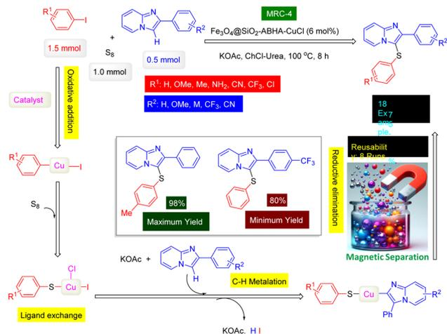
**Scheme 4**  $\text{Fe}_3\text{O}_4@\text{SiO}_2\text{-ABHA-CuCl}$  nanomaterial (**MRC-4**) catalyzed synthesis of diaryl sulfides infused with intricate imidazo[1,2-*a*]pyridine scaffolds from S<sub>8</sub>.
