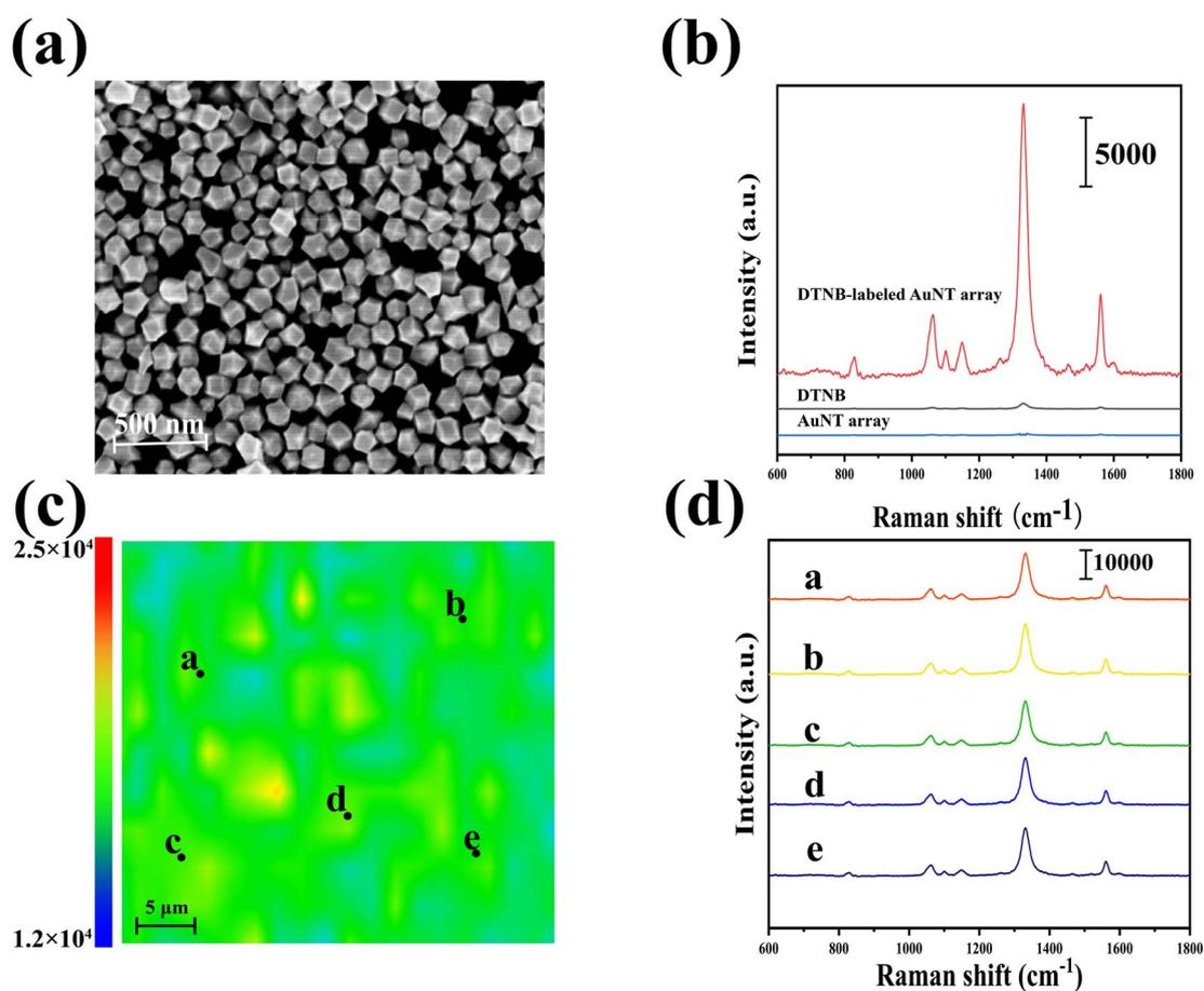
Fig. 3 (a) SEM image of an AuNT array, (b) SEM image of an AuNT array, (b) SERS spectra of DTNB ( $10^{-2}$  M), DTNB ( $10^{-8}$  M)-labeled AuNT array and AuNT array, (c) SERS mapping of the DTNB ( $10^{-8}$  M)-AuNT array, (d) SERS spectra when 5 different points (a–e) were arbitrarily selected on the DTNB ( $10^{-8}$  M)-AuNT array.
