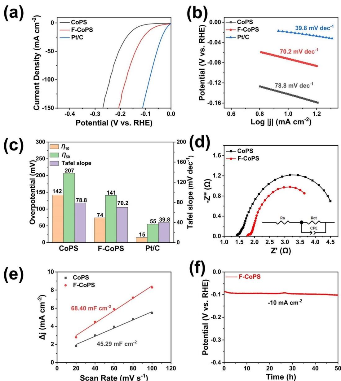
Fig. 5 (a) LSV curves, (b) Tafel slopes, (c) summary of the overpotentials and Tafel slopes of CoPS, F-CoPS and Pt/C catalysts, (d) EIS spectra of CoPS and F-CoPS, (e)  $C_{dl}$  values of CoPS and F-CoPS, and (f) chronopotentiometric curves of F-CoPS for the HER in 1 M KOH solution.
