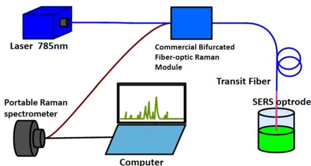
Fig. 2 Schematic for back scattered SERS measurements of the setup.
