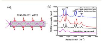
Fig. 5 (a) Evanescent field in optical fibers. (b) SERS spectra of the evanescent wave fiber SERS probe with 500 nm polystyrene spheres deposited with 27 nm, 30 nm and 33 nm silver film thicknesses to detect in 4-ATP solutions with a concentration of  $10^{-6}$  M and optical fiber background Raman spectrum.
