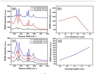
Fig. 6 (a) SERS spectra of  $10^{-6}$  M 4-ATP solutions measured using evanescent wave fiber SERS probes fabricated with different core diameters of ECFs. (b) Relationship between SERS intensity for the peak at 1079 cm $^{-1}$  and core diameters. (c) SERS spectra for  $10^{-6}$  M 4-ATP solutions measured using probes with different sensing lengths of ECFs. (d) Relation between the SERS intensity of the peak at 1079 cm<sup>-1</sup> and sensing lengths.
