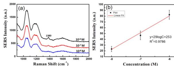
Fig. 9 (a) SERS spectra obtained using evanescent wave fiber SERS probes for thiram aqueous solutions. (b) Linearity analysis of thiram aqueous solutions with concentrations ranging from  $10^{-8}$  to  $10^{-6}$  M.
