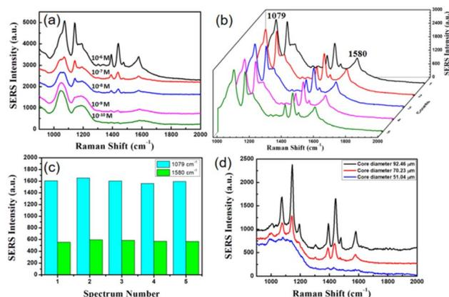
Fig. 7 (a) SERS spectra of 4-ATP solutions with concentrations of  $10^{-6}$  to  $10^{-10}$  M, obtained with evanescent wave fiber SERS probes; (b) SERS spectra of 4-ATP solutions with a concentration of  $10^{-6}$  M measured using 5 probes prepared under same process; (c) SERS intensities for peaks at  $1079\text{ cm}^{-1}$  and  $1580\text{ cm}^{-1}$ ; (d) Raman signal of the evanescent wave fiber SERS probes of different core diameters submerged in  $10^{-6}$  M 4-ATP solution.
