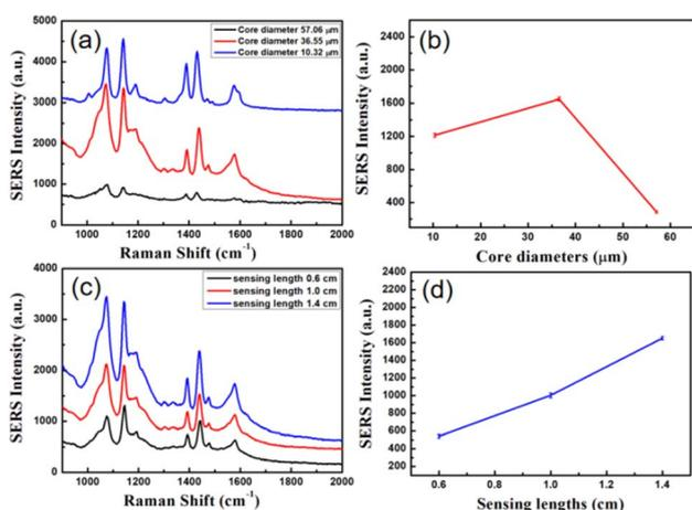
Fig. 6 (a) SERS spectra of  $10^{-6}$  M 4-ATP solutions measured using evanescent wave fiber SERS probes fabricated with different core diameters of ECFs. (b) Relationship between SERS intensity for the peak at  $1079\text{ cm}^{-1}$  and core diameters. (c) SERS spectra for  $10^{-6}$  M 4-ATP solutions measured using probes with different sensing lengths of ECFs. (d) Relation between the SERS intensity of the peak at  $1079\text{ cm}^{-1}$  and sensing lengths.
