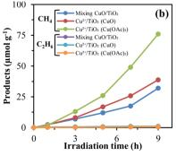
Fig. 3 (a) Effect of Cu sources on the photocatalytic methane production from acetic acid solution, and (b) comparison of hydrocarbon production rates under visible light (405 nm).
