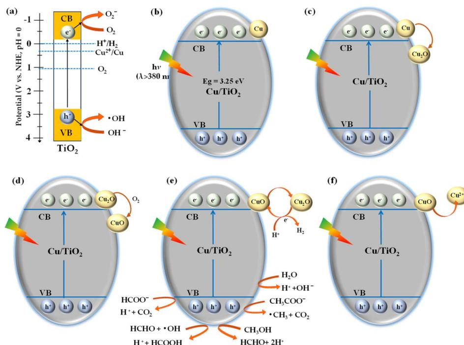
Fig. 7 Mechanism for (a) oxygen reduction, and hydroxide ion oxidation and (b–f) photocatalytic hydrocarbon and H<sub>2</sub> production.
