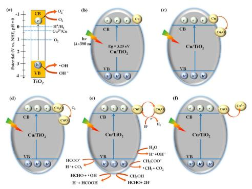
Mechanism for (a) oxygen reduction, and hydroxide ion oxidation and (b-f) photocatalytic hydrocarbon and H<sub>2</sub> production.
