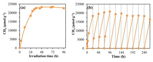
Fig. 2 (a) Effect of irradiation time on Cu/TiO<sub>2</sub> photocatalytic CH<sub>4</sub> production, and (b) stability test results of CH<sub>4</sub> production.
