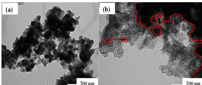
Fig. 5 TEM images of Cu/TiO<sub>2</sub> (a) before and (b) after 3 hours of irradiation.
