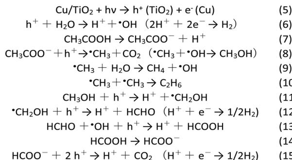
Scheme 1 Reaction mechanism for the hydrocarbon production from acetic acid.<sup>47,70,71</sup>
