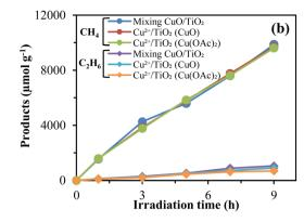
Fig. 1 (a) Effect of Cu sources on the photocatalytic methane production from acetic acid solution, and (b) comparison of hydrocarbon production rates under UV light (365 nm) irradiation.
