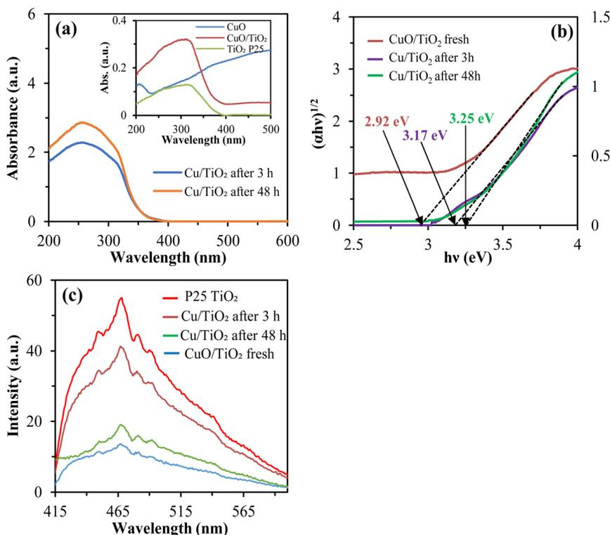
Fig. 6 (a) DRS spectra, (b) Tauc-plot and (c) PL spectra of the studied catalysts.
