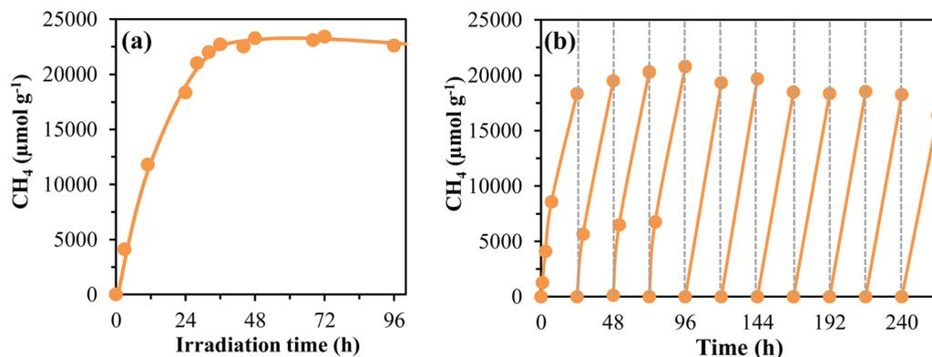
Fig. 2 (a) Effect of irradiation time on Cu/TiO<sub>2</sub> photocatalytic CH<sub>4</sub> production, and (b) stability test results of CH<sub>4</sub> production.
