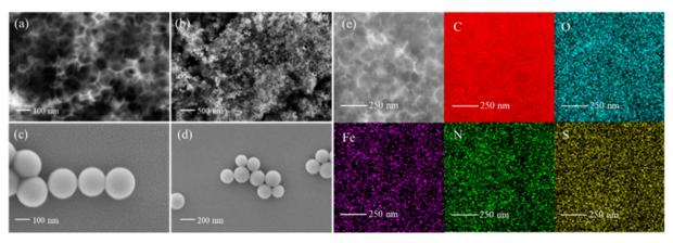
Fig. 1 SEM images of (a and b) FeSNC and (c and d) SiO<sub>2</sub>; (e) elemental distribution of FeSNC.
