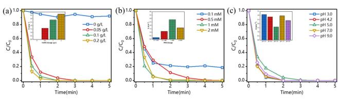
Fig. 4 Kinetic curves of BPA degradation and apparent rate constant ( $k_{obs}$ ) by FeSNC-PMS system with (a) different catalyst dosage, (b) different PMS concentration and (c) different initial pH. Experimental conditions: [BPA]<sub>0</sub> = 20 mg L<sup>-1</sup>, [PMS]<sub>0</sub> = 1 mM, [catalyst]<sub>0</sub> = 0.10 g L<sup>-1</sup>, initial pH 4.2.
