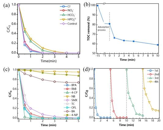
Fig. 7 (a) Kinetic curves of BPA degradation by FeSNC-PMS system in the presence of different coexisting anions; (b) TOC removal efficiency in FeSNC-PMS system. (c) Kinetic curves of FeSNC-PMS system for degradation of different organic pollutants; (d) cycling stability experiments of FeSNC-PMS system for BPA degradation.
