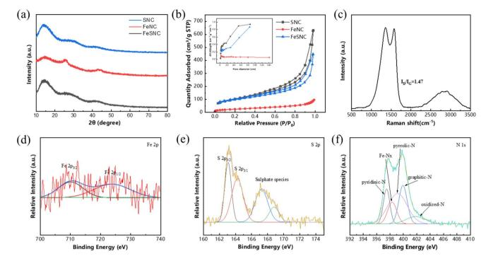
Fig. 2 (a) XRD pattern of SNC, FeNC and FeSNC; (b) N<sub>2</sub> adsorption—desorption isotherms of SNC, FeNC and FeSNC; (c) Raman spectra of FeSNC; high-resolution XPS spectrum of (d) Fe 2p, (e) S 2p and (f) N 1s of FeSNC
