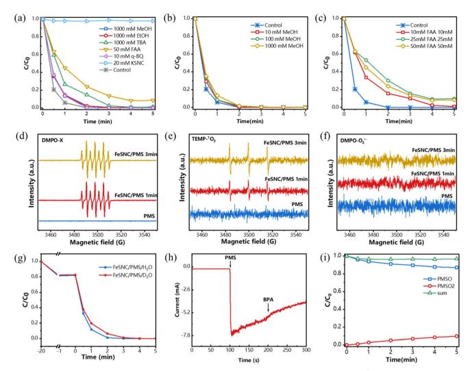
Fig. 5 (a–c) Impact of scavengers on BPA degradation in the FeSNC/PMS system; EPR analysis for DMPO-X (d),  $^{1}O_{2}$  (e), and  $O_{2}$  (f) detection of FeSNC/PMS system; (g) BPA degradation efficiency in different solvents; (h) amperometric I-t curves upon the addition of PMS and BPA; (i) PMSO loss and PMSO<sub>2</sub> production in the FeSNC/PMS system.
