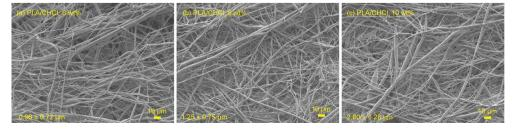
Fig. 1 FE-SEM images of the PLA fibers obtained from the PLA/CHCl<sub>3</sub> solutions with various PLA concentrations of (a) 6 wt%, (b) 8 wt%, and (c) 10 wt%.
