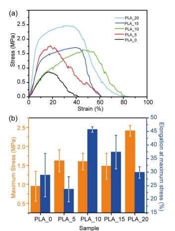
Fig. 7 (a) Stress-strain curves and (b) mechanical properties of PLA webs prepared from different PLA solutions.
