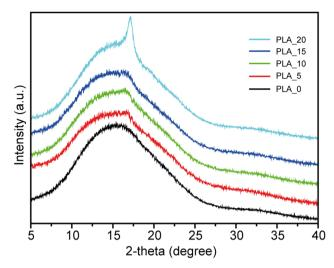
Fig. 4  $\,$  XRD patterns of the PLA fibers obtained from various CHCl $_{\rm 3}/$  DMF mixture solutions.
