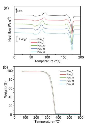
Fig. 5 (a) DSC and (b) TGA curves of the PLA fibers prepared from 10 wt% PLA solutions with different weight ratios of CHCl $_3$ /DMF.
