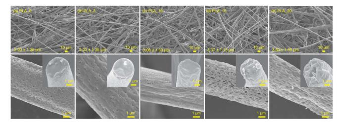
Fig. 2 FE-SEM images of surface morphology and cross-section of the PLA fibers obtained from the 10 wt% PLA solutions with various CHCl<sub>3</sub>/DMF ratios of (a) PLA\_0, (b) PLA\_5, (c) PLA\_10, (d) PLA\_15, and (e) PLA\_20.
