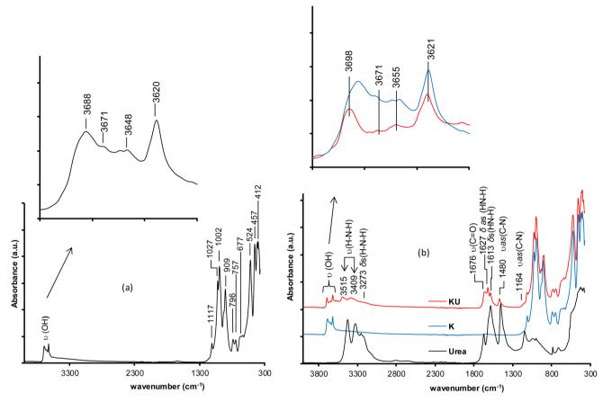
Fig. 3 FTIR spectra of (a) raw kaolinite; (b) urea, kaolinite (K) and urea-intercalated kaolinite (KU). v: Stretching vibrations; v as: asymmetric stretching vibrations; v as: asymmetric bending vibrations; v as: asymmetric bending vibrations; v as: asymmetric bending vibrations.
