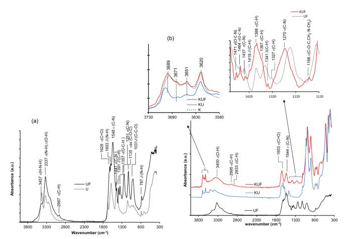
Fig. 5 FTIR spectra of (a) free poly(urea-formaldehyde) (UF) and urea (U); (b) urea-intercalated kaolinite (KU), and intercalated kaolinite-poly(urea-formaldehyde) (KUF). v: Stretching vibrations;  $v_{as}$ : asymmetric stretching vibrations;  $\delta$ : bending vibrations.
