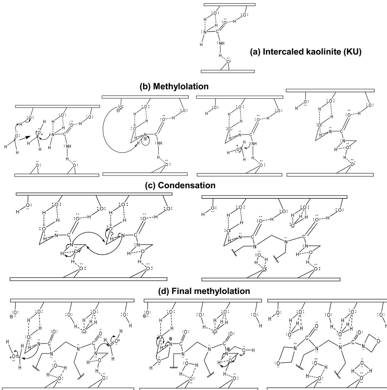
Fig. 8 Proposed mechanism for the *in situ* polymerization of urea-formaldehyde in kaolinite interstitial space: (a) urea-intercalated kaolinite; (b) first methylation; (c) condensation; (d) final methylation.
