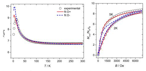
Fig. 7 Magnetic data for compound 1. Temperature dependence of the effective magnetic moment and the isothermal magnetizations measured at T = 2 and 5 K. The empty circles represent the experimental data points and the lines represent the best fits calculated by using eqn (1) and (3) with parameters listed in Table S3.‡ Full red line represents the best fits calculated for the positive D parameter. The dashed blue line represents the best fits calculated for the negative D parameter.
