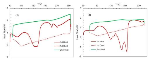
Fig. 4 Differential scanning calorimetry (DSC) heating and cooling curves for 1 and 2
