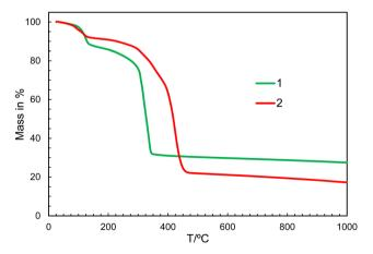
Fig. 3 Thermogravimetric curves (TGA) for 1 and 2 (heating rate 5 K  $\text{min}^{-1}$  under  $N_2$  atmosphere).
