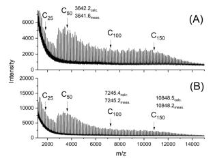
Fig. 2 MALDI TOF mass spectra of cyclic PLAs prepared with BuSnSPF at 140 °C/2 d: (A) LA/Cat = 200/1 (no. 1A, Table 1), (B) LA/Cat = 500/1 (no. 3A, Table 1).
