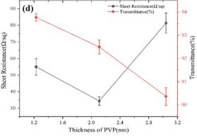
Fig. 3 SEM images of AgNWs@PVP core-shell layer structures with different PVP thicknesses and statistical plots of sheet resistance and transmittance after high-temperature sintering. (a)  $1.20 \pm 0.03$  nm, (b)  $2.11 \pm 0.01$  nm, (c)  $3.03 \pm 0.01$  nm, (d) statistical plots.
