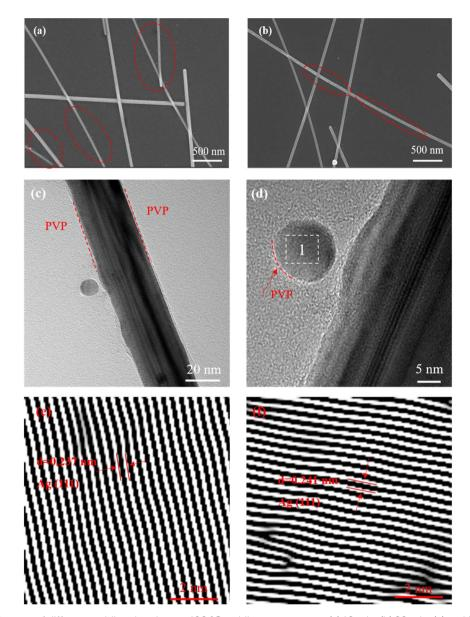
Fig. 5 SEM and TEM images of different welding durations at 190 °C welding temperature. (a) 10 min, (b) 20 min, (c) and (d) 10 min-TEM, (e) and (f) lattice fringes in region 1.
