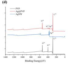
Fig. 1 (a) SEM image of AgNWs before centrifugal cleaning. (b) SEM images of AgNWs after centrifugal cleaning. (c) TEM images of AgNWs used in this work. (d) XPS images of AgNWs before and after centrifugation and XPS images of PVP.
