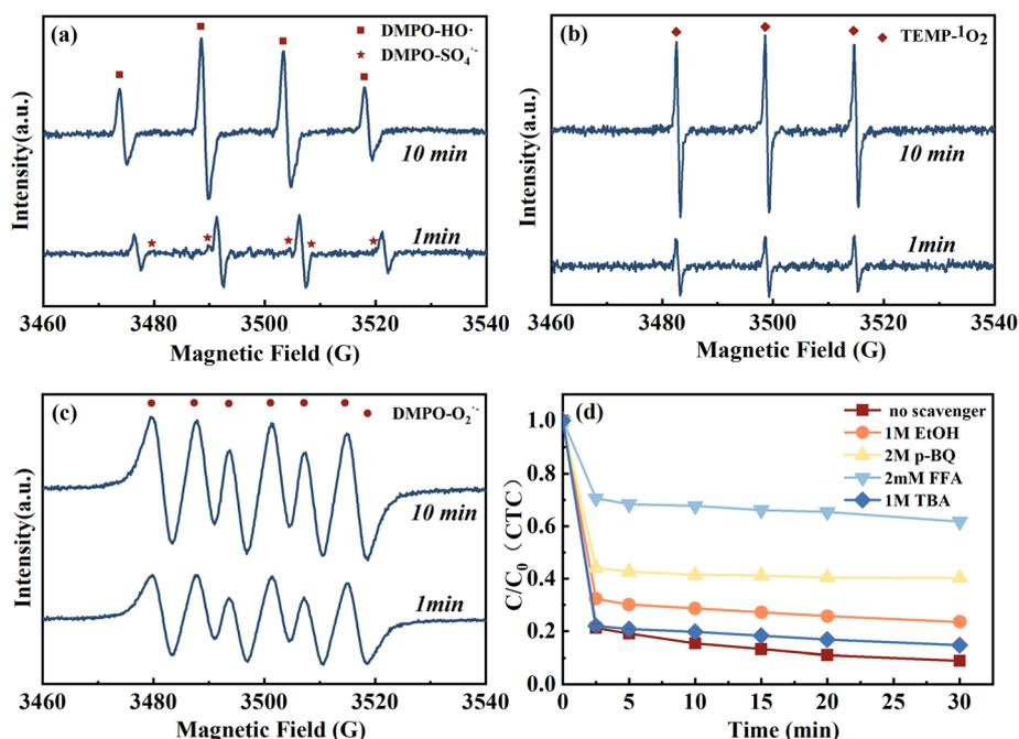
Fig. 6 Effect of radicals quenching on degradation of CTC and EPR spectra in MnFeCu-LDH/GO activating PMS system, (a) present  $\cdot\text{OH}$  and  $\text{SO}_4^{\cdot-}$ , (b) and (c) present  $^1\text{O}_2$  and  $\text{O}_2^{\cdot-}$ , respectively, (d) present degradation efficiency of CTC under different quencher.
