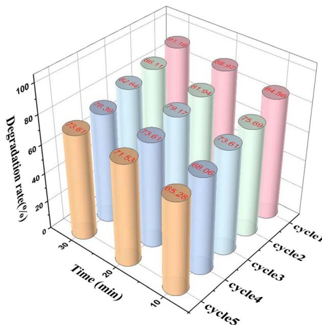
Fig. 4 The reusability of MnFeCu-LDH/GO (reaction conditions: initial CTC concentration = 10 mg L<sup>-1</sup>, catalyst dosage = 0.2 g L<sup>-1</sup>, PMS dosage = 0.2 g L<sup>-1</sup>, reaction temperature = 25 °C and initial pH = 7).
