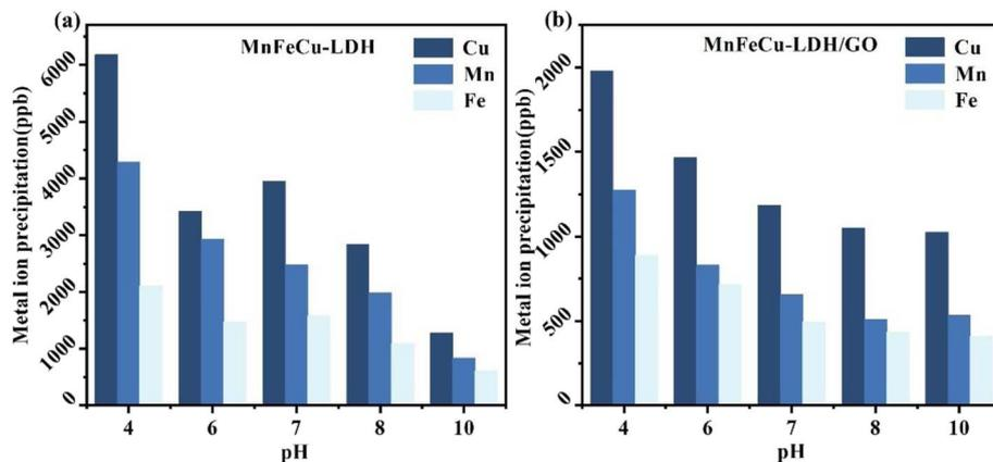
Fig. 5 Leaching of ions after the reactions at different initial pH of MnFeCu-LDH/GO, (a) for MnFeCu-LDH, (b) for MnFeCu-LDH/GO (reaction conditions: initial CTC concentration = 10 mg L<sup>-1</sup>, catalyst dosage = 0.2 g L<sup>-1</sup>, PMS dosage = 0.2 g L<sup>-1</sup> and reaction temperature = 25 °C).
