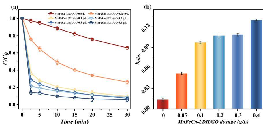
Fig. 2 The degradation efficiency of CTC at different dosage MnFeCu-LDH/GO, (a) present removal rate, (b) present obvious rate constant of degradation kinetics ( $k_{\text{obs}}$ ) (catalyst dosage: 0.05–0.4 g L<sup>-1</sup>, PMS dosage: 0.2 g L<sup>-1</sup>, reaction temperature = 25 °C).
